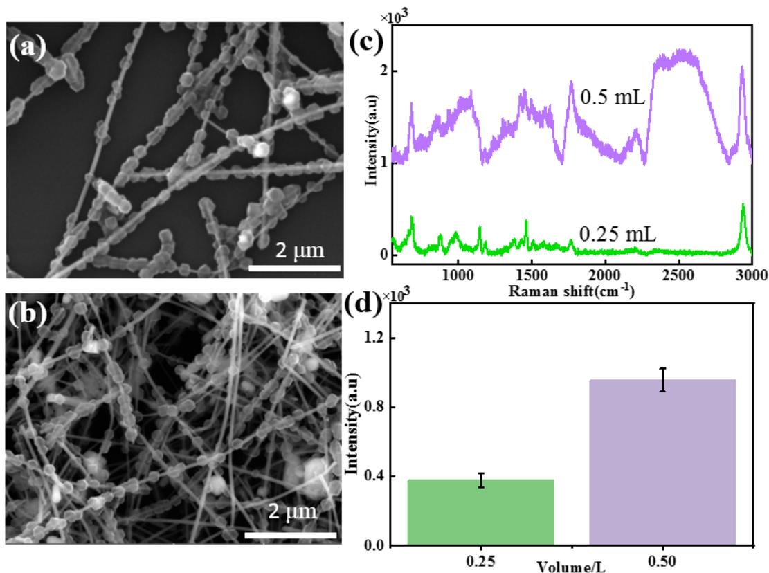
**Fig. 2** SEM images of the Ag NWs@ZIF core-shell nanochains prepared with volumes of (a) 0.25 mL and (b) 0.5 mL of Ag NWs. (c) SERS spectra of methanethiol gas molecules ( $10^{-4}$  M) collected on Ag NWs@ZIF substrates with different volumes of Ag NWs. (d) The corresponding histogram of the SERS intensity at  $2931\text{ cm}^{-1}$ .
