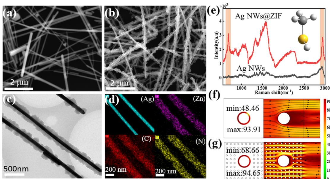
**Fig. 1** (a) SEM micrographs of the synthesized Ag nanoparticles and (b) Ag NWs@ZIF. Scale bar: 2  $\mu\text{m}$ . (c) TEM micrographs of Ag NWs@ZIF. Scale bar: 500 nm. (d) The corresponding energy-dispersive X-ray spectroscopy (EDX) elemental mapping of Ag, Zn, C and N. Scale bar: 200 nm. (e) SERS spectra of (red) Ag NWs@ZIF and (black) Ag-only platforms for adsorbing gaseous methanethiol. The velocity distribution pattern for (f) Ag NW substrates and (g) Ag NWs@ZIF structures.
