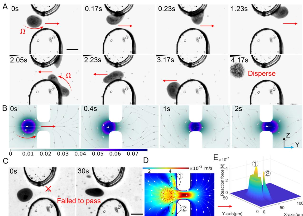
**Fig. 6** Magnetic nanoparticle swarm crosses the simulated cell gap. (A) Magnetic nanoparticle swarm creeps back and forth through the cell interstices by climbing on the wall. The scale bar is 10  $\mu\text{m}$ . (B) The simulation of a swarm crosses the narrow gap. (C) Magnetic nanoparticle swarm cannot get right through the slit. The scale bar is 10  $\mu\text{m}$ . (D) Simulation of a swarm unable to pass directly through a slit. (E) Fluid and wall reaction forces due to swarm rotation.
