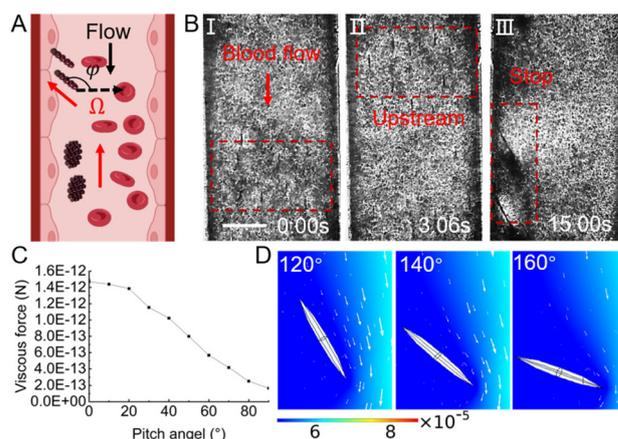
**Fig. 5** Motion control of swarms in the blood flow. (A) The illustration of upstream movement and targeted stopping of magnetic nanoparticle swarm. (B) The upstream movement and targeted stopping of magnetic nanoparticle swarm in pulsatile blood flow. The scale bar is 100  $\mu\text{m}$ . (C) Viscous drag versus magnetic field pitch angle. (D) Simulation of the swarm motion under different magnetic field yaw angles.
