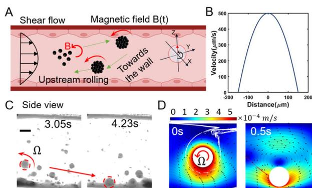
**Fig. 4** Lateral effects generated by the high-speed rotation of magnetic nanoparticle swarm. (A) The illustration of the swarms dragging themselves to the wall by high-speed rotation. (B) Flow velocity distribution along the diameter of the experimental blood vessel. (C) Magnetic nanoparticle swarm rotating towards the wall. The scale bar is 50  $\mu\text{m}$ . (D) Simulation of flow field distribution around the swarm.
