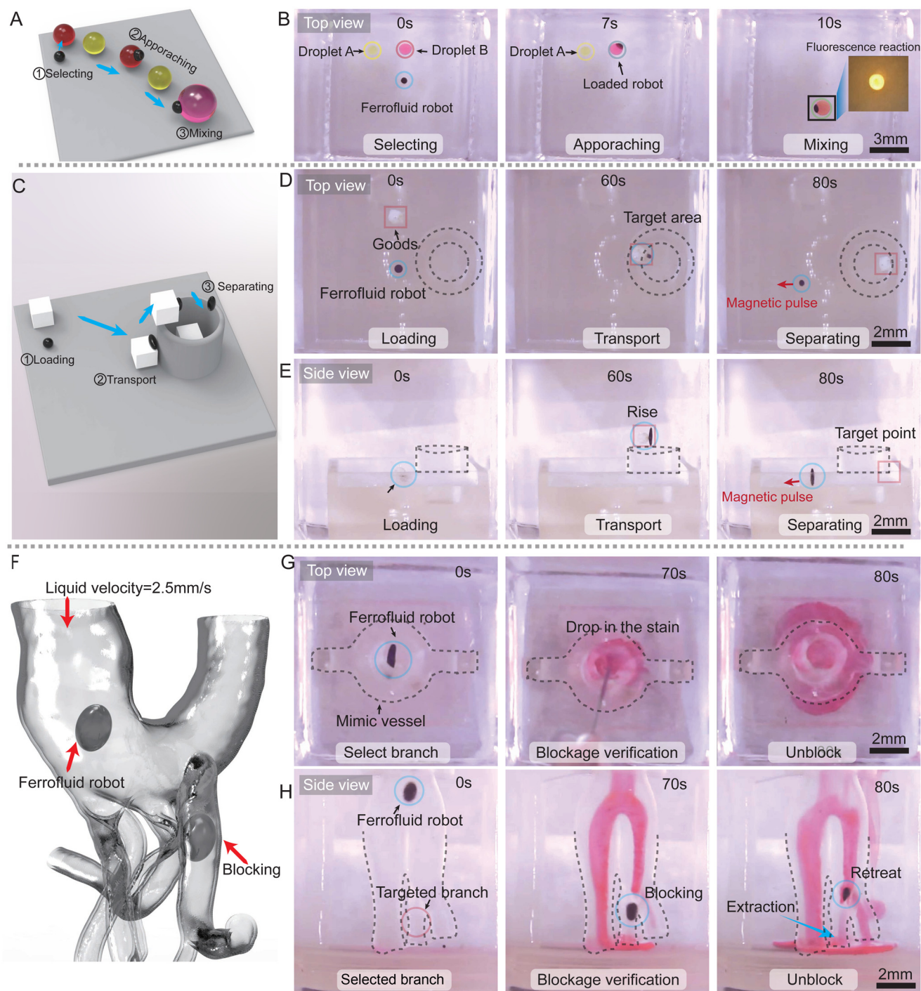
Fig. 7 Experimental validation of multifunctionality in ferrofluidic robots. (A) Conceptual illustration of a ferrofluidic robot employed for controlled chemical micro-reactions via droplet mixing. (B) The process and fluorescence imaging results of a fusion reaction, orchestrated by a ferrofluidic robot, between droplets containing disparate solvents. (C) Schematic representation of a ferrofluidic robot purposed for micro-operation. (D) Top view and (E) primary view of a ferrofluidic robot controlling and conveying goods to a designated area, demarcated by the black dashed contour line. (F) Conceptual depiction of a ferrofluidic robot for selective blood vessel occlusion. (G) Top view and (H) primary view of the experimental procedure illustrating controllable blood vessel blockage facilitated by a ferrofluidic robot.
