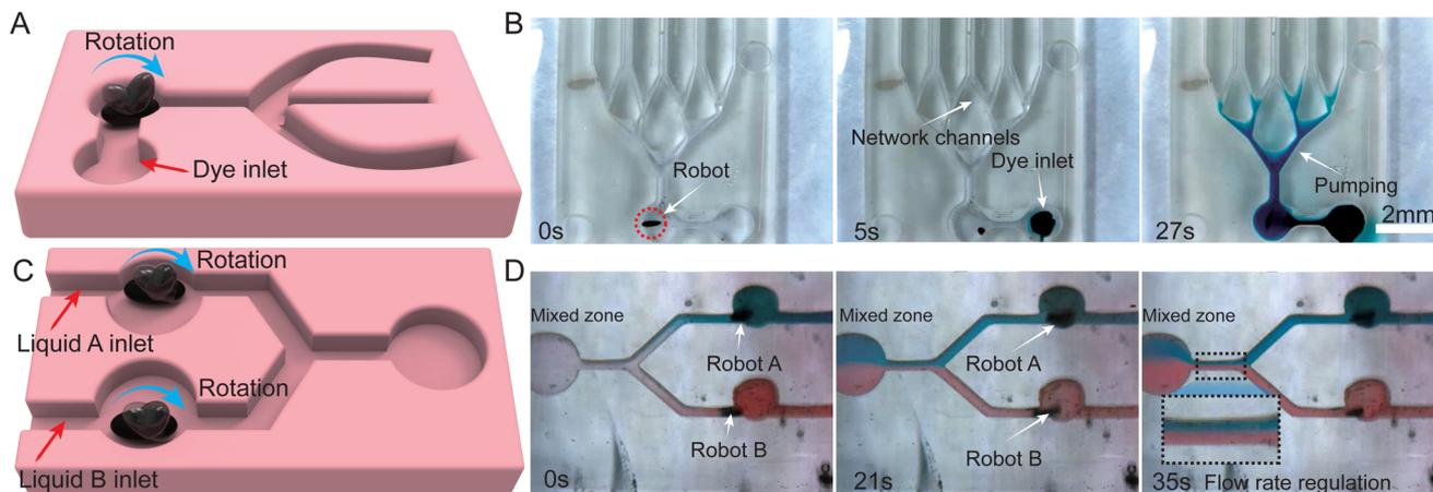
**Fig. 5** Deformed ferrofluidic robots as a microfluidic inducer. (A) Conceptual diagram depicting a deformed ferrofluidic robot functioning as a micropump. (B) Experimental evaluation of a deformed ferrofluidic robot pumping dye in network channels. (C) Schematic representation of deformed ferrofluidic robots employed as mixers. (D) Experimental exploration of two deformed ferrofluidic robots collaborating to mix dyes in a Y-shaped channel.
