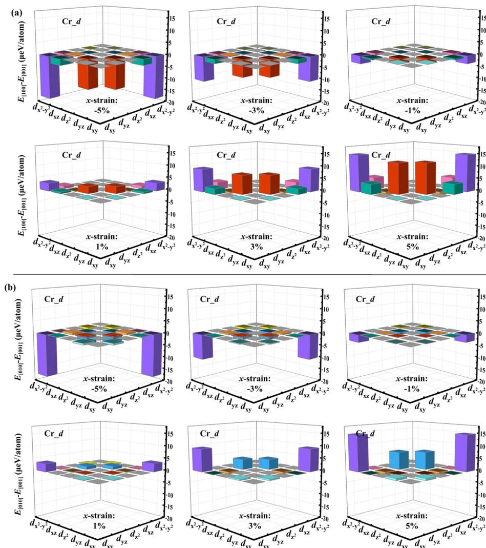
**Fig. 5** The contribution to MAE from the SOC interaction between different d orbital channels for Cr atoms under different uniaxial x strains along the [100] (a) and the [010] (b) directions. The energy is the reference along the [001] direction.
