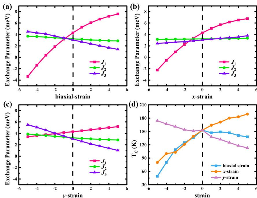
Fig. 6 Variation of exchange parameters with biaxial strain (a), uniaxial strain in the x-direction (b), and uniaxial in the y-direction (c), respectively. (d) The changes of  $T_C$  at different strains.
