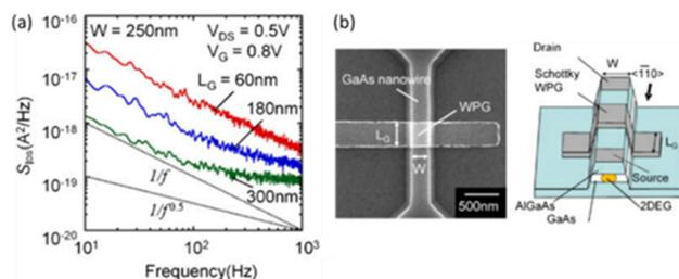
**Fig. 19** (a) Current noise power-spectral densities of Schottky wrap-gate (WPG) GaAs/AlGaAs NW transistors with  $W = 250 \text{ nm}$  and varying  $L_G$ . (b) Top view and schematic cross-section. Adapted from ref. 64 with permission. Copyright 2011 Institute of Physics.
