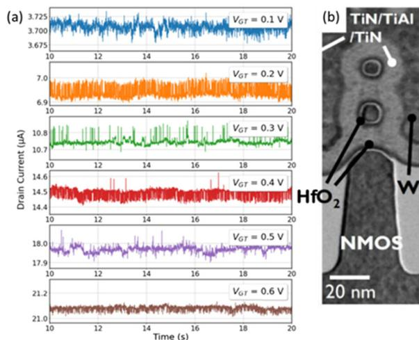
**Fig. 25** Gate-to-threshold voltage dependence of  $I_{DS}$  at 295 K for a GAA NW nFET with  $L \approx 25$  nm, 8 nm diameter, and 1.8 nm  $\text{HfO}_2/1$  nm gate dielectric; a transmission-electron-microscope image of the structure is shown in (b).  $V_{DS} = 50$  mV;  $V_{GT} \equiv V_{GS} - V_{TH}$ . Note that each value of  $V_{GT}$  has a different y-axis scale. Adapted from ref. 74 with permission. Copyright 2021 Institute of Electrical and Electronics Engineers.
