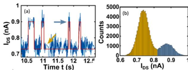
Fig. 22 (a) RTN at a temperature of 150 K in a vertical InAs/InGaAsSb/GaSb NW tunnel FET with a 20 nm InAs channel diameter and Al<sub>2</sub>O<sub>3</sub>/HfO<sub>2</sub> gate dielectric with effective oxide thickness of 1.4 nm. (b) Histograms of current values measured in the higher conductivity (gold) and lower conductivity (blue) states of the device, corresponding to the respective arrows in (a). Adapted from ref. 69 with permission. Copyright 2017 American Chemical Society.
