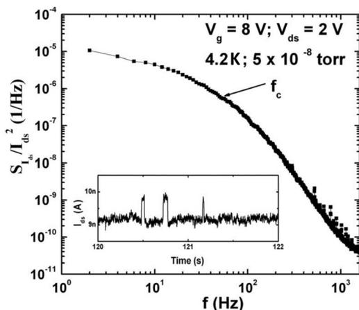
Fig. 5 Lorentzian noise power spectrum for a ZnO NW exhibiting random telegraph noise, RTN, at a temperature of 4.2 K. The corner frequency  $f_c$  is  $\sim 18$  Hz. The inset plots current *vs.* time. Reproduced from ref. 62 with permission. Copyright 2007 American Institute of Physics.
