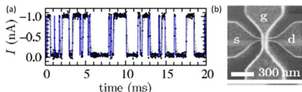
Fig. 23 (a) RTN for a silicon NW on a silicon-on-insulator (SOI) wafer with length of 200 nm and width of 30 nm with SiO<sub>2</sub> gate oxide thickness of 24 nm.  $V_{GS} = 0.5$  V,  $V_{DS} = -6$  mV. (b) Top view of NW. Adapted from ref. 59 with permission. Copyright 2006 Springer.
