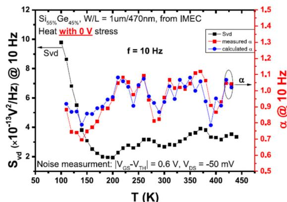
**Fig. 6** Noise magnitude (left y-axis) and measured and predicted values of  $\alpha = -\partial \ln S_{V_d} / \partial \ln f$  vs. temperature (right y-axis) for a SiGe pMOSFET with SiO<sub>2</sub>/HfO<sub>2</sub> gate dielectric. Predicted  $\alpha$  values are derived from the  $S_{V_d}$  vs.  $T$  curve measured before bias-temperature stress, using eqn (5) of the text. Reproduced from ref. 133 with permission. Copyright 2016 Institute of Electrical and Electronics Engineers.
