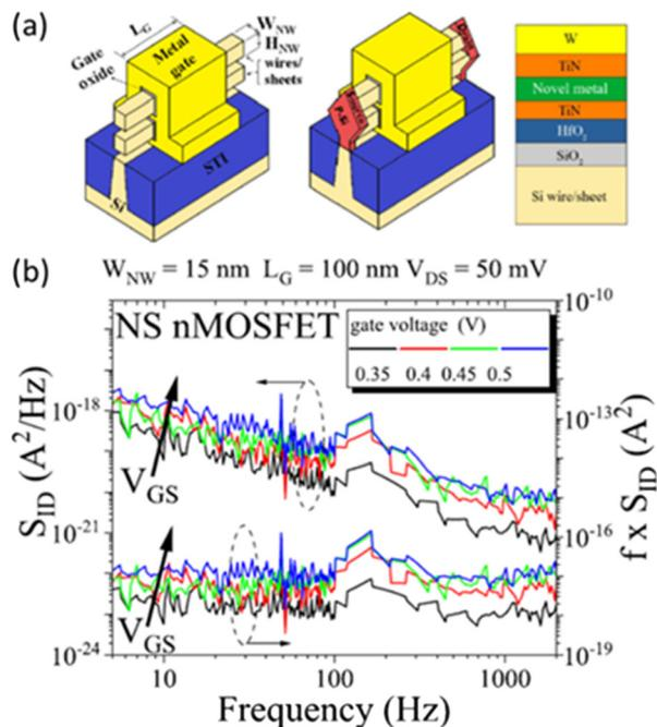
**Fig. 24** (a) Schematic diagrams of gate-all-around GAA nFETs with two vertically stacked Si nanosheets. (b) Drain current noise power spectral density (left y-axis) and normalized power spectral density (right y-axis) as a function of frequency for a 15 nm nanosheet width device at different gate voltages. Adapted from ref. 72 with permission. Copyright 2020 Institute of Electrical and Electronics Engineers.
