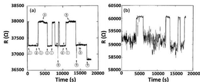
**Fig. 14** (a) Resistance vs. time at  $T = 70 \text{ mK}$  for an  $\sim 8 \text{ nm}$  thick Bi film with  $L = 10 \mu\text{m}$  and  $W = 4 \mu\text{m}$ . Numbers denote different fluctuators. (b) Resistance vs. time at 250 mK for a 1 nm thick Pt film with  $L = 7 \mu\text{m}$  and  $W = 5 \mu\text{m}$ . Adapted from ref. 54 with permission. Copyright 1987 Institute of Physics.
