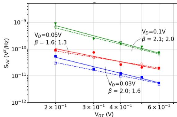
**Fig. 28** Gate-voltage dependence of  $S_{V_d}$  at  $V_{DS} = 30$  mV, 50 mV, and 100 mV for as-processed (closed symbols, solid lines) and irradiated (open symbols, dashed lines) GAA NW nFETs. The device was irradiated to 1 Mrad(SiO<sub>2</sub>) with 10 keV X-rays at  $V_{GS} = 0.5$  V. Reproduced from ref. 74 with permission. Copyright 2021 Institute of Electrical and Electronics Engineers.
