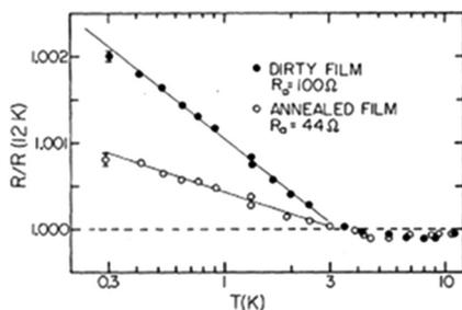
**Fig. 10** Relative resistance vs. temperature for an as-processed, sputtered AuPd thin film ("dirty") with sheet resistance of  $100 \Omega \square^{-1}$  and an otherwise identical film annealed for 24 h in Ar at  $300^\circ\text{C}$  with sheet resistance of  $44 \Omega \square^{-1}$ . Lines are best fits to the data. Reproduced from ref. 7 with permission. Copyright 1980 The American Physical Society.
