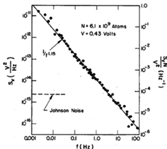
**Fig. 1** Excess voltage-noise power spectral density  $S_V$  as a function of frequency  $f$  for a Pt nanowire (NW) fabricated *via* substrate step lithography. The Johnson (thermal) noise background has been subtracted. The size and voltage normalized noise,  $S_V N/V^2$  is shown on the right-h and y-axis, with  $N = N_A$ . Reproduced from ref. 51 with permission. Copyright 1983 The American Physical Society.
