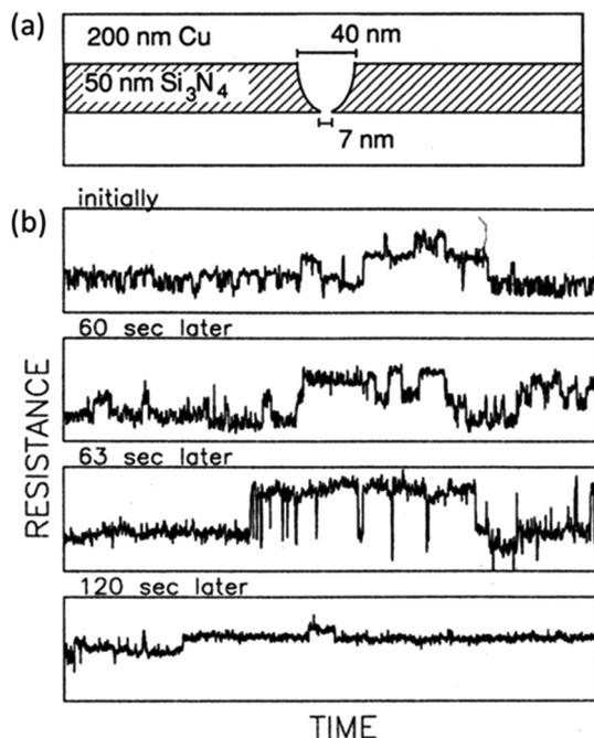
**Fig. 18** (a) Schematic diagram of Cu nanobridge and (b) resistance vs. time snapshots (0.2 s each) at 300 K, illustrating the time evolution of defect-induced scattering in these structures at room temperature. Reproduced from ref. 57 with permission. Copyright 1989 The American Physical Society.
