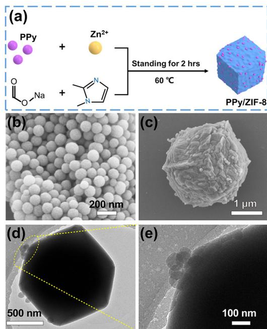
**Fig. 1** Fabrication and morphological characterization. (a) Schematic illustrating the preparation of PPy/ZIF-8 through the *in situ* encapsulation method. SEM images of (b) PPy NPs and (c) PPy/ZIF-8. (d) TEM image of PPy/ZIF-8. (e) An enlarged view image of (d).
