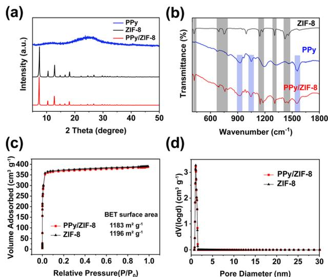
**Fig. 2** Structural characterization. (a) Powder XRD patterns and (b) FTIR spectra of PPy NPs, ZIF-8, and PPy/ZIF-8. (c)  $N_2$  adsorption-desorption isotherms and (d) pore size distributions of ZIF-8 and PPy/ZIF-8 based on the NLDFT method.
