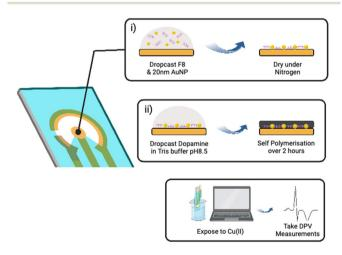
Fig. 3 DNAzyme based electrochemical biosensor for Cu(II) is prepared by drop casting DNAzyme/substrate complex and rate enhancing Au NPs to the surface of electrode (i) followed by addition of dopamine and self-polymerisation resulting in PDA coating. (ii) Sensor is prepared within 2 hours after which Cu(II) detection can be performed using differential pulse voltammetry (DPV).
