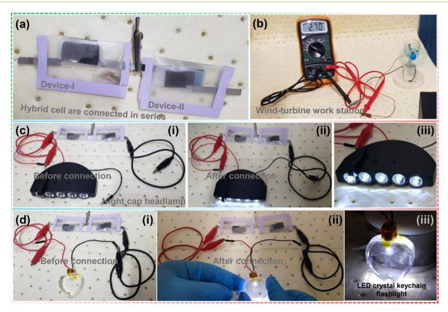
Fig. 5 Photographic images of practical applications: (a) two AHCs connected in series to extend the potential, packaged with transparent parafilm. (b) Wind energy conversion to charge the designed AHCs. (c) Cap lights on night-cap LED headlamp before and after connection. (d) LED crystal key flashlight before and after connection to the AHCs.
