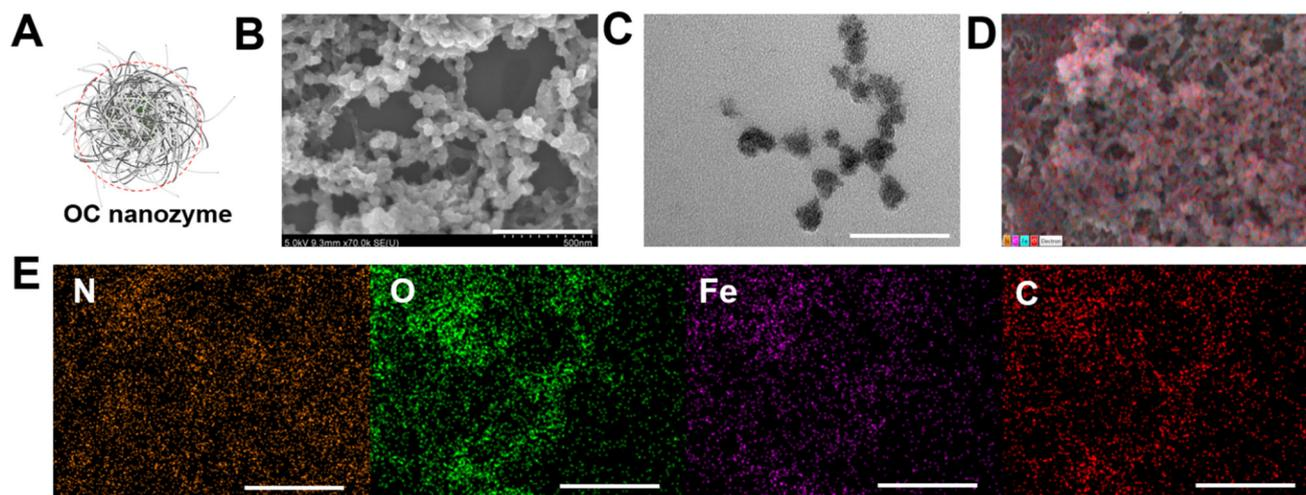
**Fig. 1** Morphological analysis of the OC nanozyme. (A) illustrates a schematic of the OC nanozyme and its spherical structure, (B) SEM image (scale bar: 500 nm), (C) Bright-field TEM image (Scale: 150 nm), (D) EDS scanning spot from SEM image, (E) EDS mapping image with the elements, carbon, oxygen, nitrogen, and iron (Scale bar = 1  $\mu$ m).
