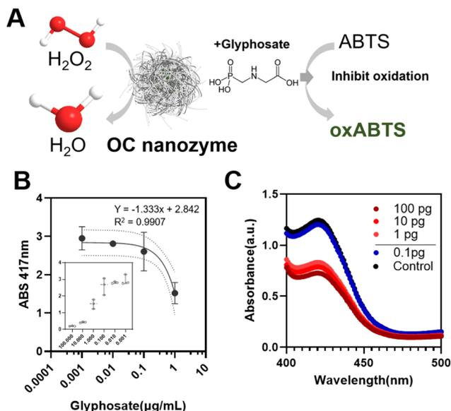
**Fig. 4** Colorimetric glyphosate detection through OC nanozyme- $\text{H}_2\text{O}_2$ -ABTS assay. (A) Illustrated strategy of the glyphosate detection, (B) Absorbance endpoint measurement of the glyphosate (inset graph/ $1 \text{ ng mL}^{-1}$ – $100 \text{ } \mu\text{g mL}^{-1}$ ) and the linearity analysis ( $1 \text{ ng mL}^{-1}$ – $1 \text{ } \mu\text{g mL}^{-1}$ ), x-axis: log-scaled,  $N = 3$ , (C). Absorbance spectra for the LOD measurement (black: control/without glyphosate).
