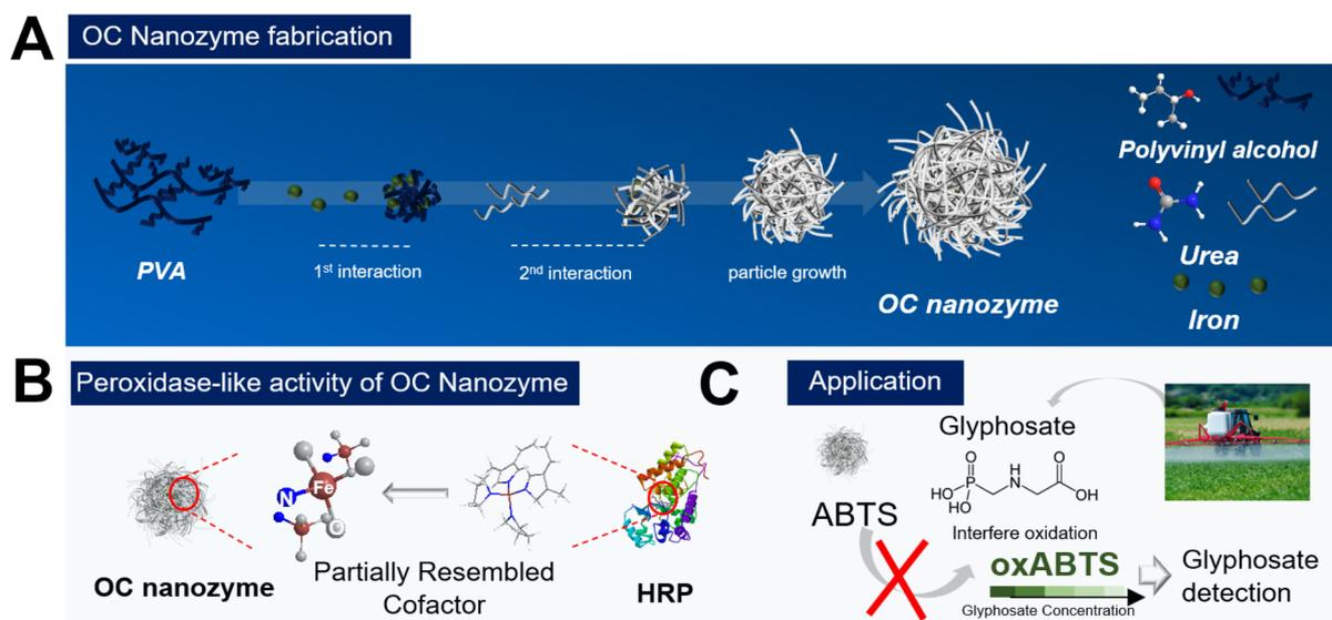
**Scheme 1** Schematic illustration of the OC nanozyme. (A) Fabrication of the OC nanozyme, (B) Partially-mimicked heme cofactor (e.g., Fe–N) containing the OC nanozyme, (C) OC nanozyme for agricultural herbicide detection.
