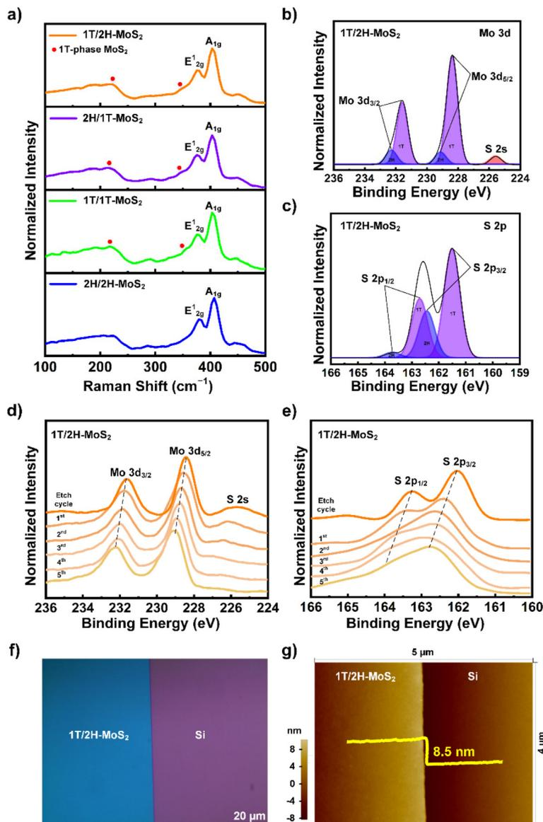
**Fig. 1** 1T/2H-MoS<sub>2</sub> characterization: (a) Raman spectroscopy and XPS surface analyses of (b) Mo 3d and (c) S 2p core peak spectra. XPS depth profile analyses of (d) Mo 3d and (e) S 2p core peak spectra. (f) OM and (g) AFM analyses of 1T/2H-MoS<sub>2</sub> on Si wafer.
