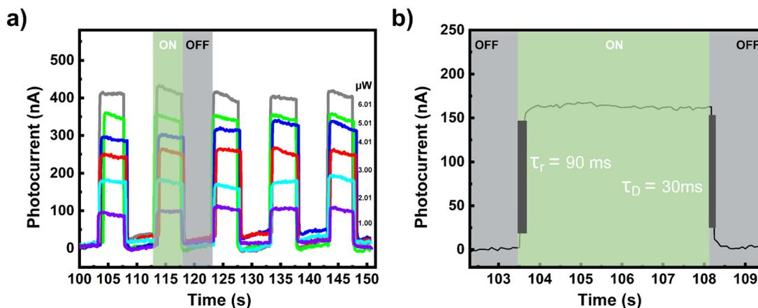
**Fig. 4** (a) Photoswitching curves for different powers of the 530 nm laser and (b) the rise and decay times according to a single ON/OFF cycle of the 1T/2H-MoS<sub>2</sub> photodetector.
