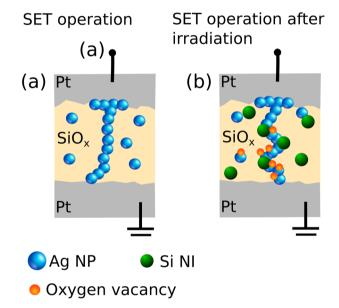
Fig. 5 Schematics of a  $SiO_x$ : Ag diffusive memristor showing (a) conductive filament in the LRS for the pristine sample before irradiation. (b) Conductive filament in the LRS for the sample after irradiation, containing Si NIs and oxygen vacancies. Both cases correspond to the positive potential applied to the top electrode.
