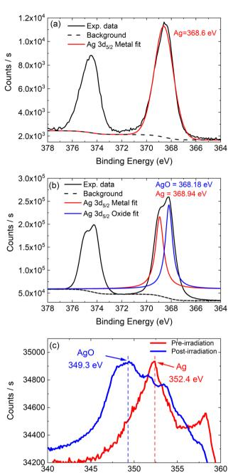
Fig. 2 (a and b) XPS spectra (black line) of Ag  $3d_{3/2}$  and  $3d_{5/2}$  peaks before (a) and after irradiation (b). The corresponding fits represent peaks for metallic Ag (red line) and silver oxide (blue line) in  $3d_{5/2}$ . (c) Auger MNN peak for Ag before (red) and after (blue) irradiation.
