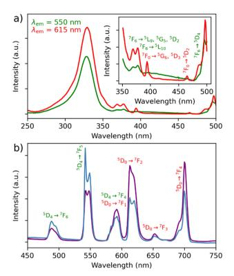
Fig. 3 (a) Excitation spectra of MSN-1 monitored at  $\lambda_{\rm em}=550$  (green) and  $\lambda_{\rm em}=615$  nm (red) recorded in the solid state at RT. Inset: magnification of the excitation spectra between 340 and 510 nm. (b) Emission spectra of MSN-1 recorded at 77 K (blue) and room temperature (violet) in the solid state with excitation at  $\lambda_{\rm em}=328$  nm. Eu<sup>3+</sup> and Tb<sup>3+</sup>-linked transitions are shown in red and green, respectively.
