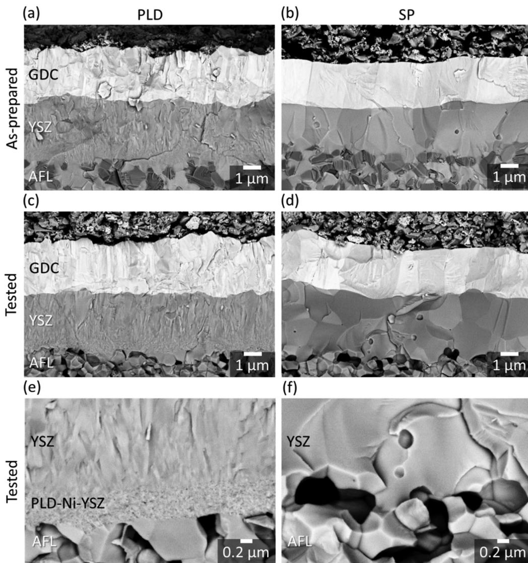
**Fig. 2** SEM backscattered electron images depicting the microstructures of the PLD cells (left column) and SP cells (right column). (a) and (b) The as-prepared cells; (c) and (d) tested cells; (e) and (f) high-magnification SEM images highlighting the YSZ/AFL interfaces of the tested PLD and SP cells, respectively.
