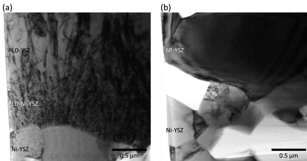
**Fig. 4** TEM images depicting the microstructures of the (a) PLD and (b) SP cells. The PLD-YSZ thin film consists of nanocolumnar grains  $\sim 100$ – $200$  nm in width, whereas the SP-YSZ layer consists of relatively larger micron-sized grains.
