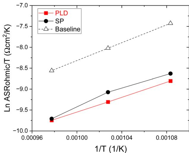
**Fig. 7** Arrhenius-type plot of the area-specific ohmic resistance comparing the performance of the PLD cell (red squares; PLD-1), the SP cell (black circles; SP-1), and a baseline sample (open triangles; no thin films included in the cell). The PLD cell shows the lowest ohmic resistance values for the entire range of temperatures investigated.
