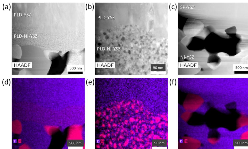
**Fig. 3** STEM-HAADF images of the tested PLD cell (a) in comparison with the SP cell (c). The corresponding STEM-EDX overlay images (Zr in purple and Ni in pink) showing the YSZ electrolyte on a Ni-YSZ nanocomposite prepared using PLD are shown below ((d) and (f)). The fine distribution of Ni and YSZ phases within the Ni-YSZ nanocomposite of the PLD cell is shown in detail in the high magnification STEM-HAADF image (b) and STEM-EDX mapping (e).
