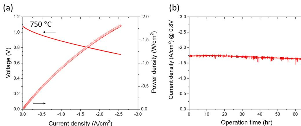
**Fig. 8** (a)  $I$ – $V$ – $P$  characteristics of anode-supported PLD cell thin film layers. (b) Short-term durability of the PLD cell at a constant potential of 0.8 V at 750 °C under 3%  $\text{H}_2\text{O}$ –97%  $\text{H}_2$  fuel gas flow.
