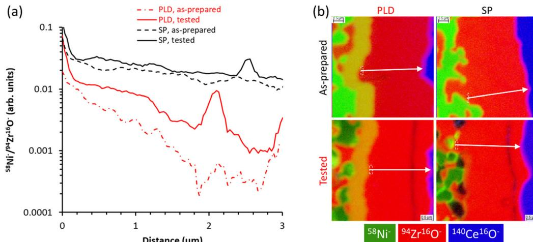
**Fig. 6** (a) Linescan profiles of the Ni/Zr ratio as extracted from the NanoSIMS mapping data shown on the right. (b) NanoSIMS mapping showing the composite images obtained from overlaying the secondary ions of  $^{58}\text{Ni}^-$  (shown in green),  $^{94}\text{Zr}^{16}\text{O}^-$  (shown in red), and  $^{140}\text{Ce}^{16}\text{O}^-$  (shown in blue). Prominent peaks in the tested samples correspond to microcracks in the specimens and are considered as measurement artefacts.
