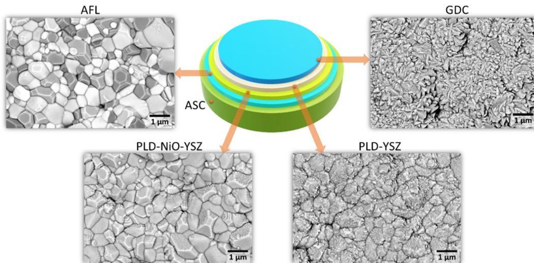
**Fig. 1** Center: schematic illustration of an anode-supported cell configuration and the representative plane-view SEM backscattered electron images of the AFL and the NiO-YSZ, YSZ, and GDC layers deposited in sequence using PLD.
