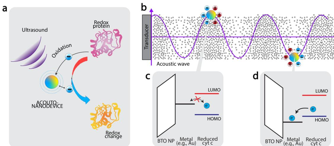
**Fig. 3** Protein oxidation by acousto-nanodevice driven under external acoustics. (a) principle of acousto-nanodevice-driven protein redox (b) The work function of the surface metal of the acousto-nanodevice oscillates under incoming acoustic waves, (c–d) a unidirectional electron transfer from protein to acousto-nanodevice is achieved because of the band alignment between the surface metal and the HOMO/LUMO levels of the protein redox center.
