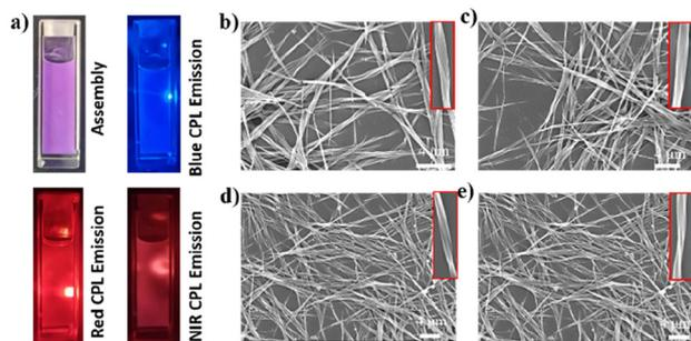
**Fig. 5** (a) Photographs of BTABA/NR/CY7, which were captured using a mobile telephone assisted by filters to avoid other emissions. (b) SEM images of BTABA assemblies. (c) SEM images of BTABA/NR assemblies. (d) SEM images of BTABA/CY7 assemblies. (e) SEM images of BTABA/NR/CY7 assemblies. [BTABA] = 5.29 mM, [NR] = 0.088 mM, [CY7] = 0.088 mM.
