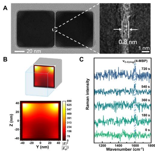
**Fig. 3** (A) High-resolution TEM image of a single Pd nanocube dimer with an enlarged view showing the gap (right). (B) Finite-difference time-domain calculation of the electric field intensity (YZ plane) inside the gap of the Pd nanocube dimer. (C) *In situ* SERS spectra of 4-mercaptobiphenyl (4-MBP) formation during Suzuki–Miyaura coupling reaction recorded at different reaction times. Reproduced from ref. 115 with permission from American Chemical Society, copyright 2022.
