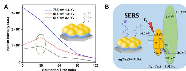
**Fig. 10** (A) Intensity of Raman peak at 1586 cm<sup>-1</sup> of 4-MBA on Ag/Cu<sub>2</sub>S hemispherical dual-shell with various excitation wavelengths and sputtering times and (B) the corresponding coupling scheme in this Ag/Cu<sub>2</sub>S/4-MBA system. Reproduced from ref. 195 with permission from American Chemical Society, copyright 2018.
