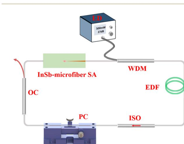
Fig. 7 The setup of a mode-locked EDF laser.
