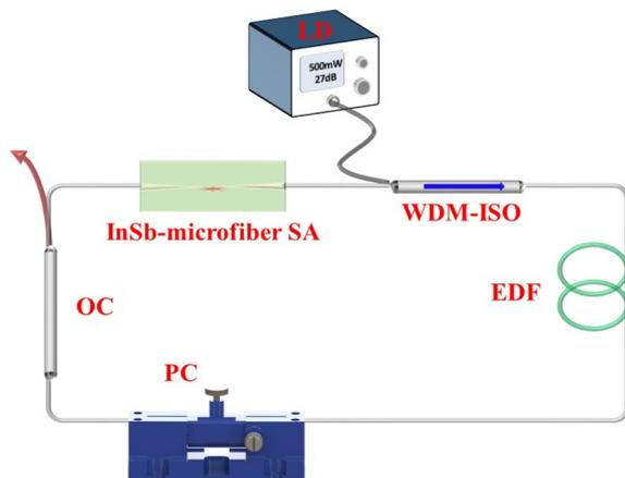
Fig. 5 The setup of the Q-switched EDF laser.
