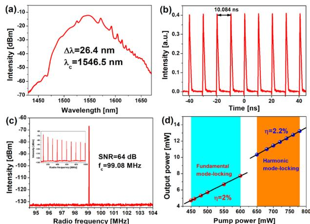
**Fig. 9** Second harmonic mode-locked experiment results: (a) optical spectra; (b) pulse sequence; (c) RF spectra; and (d) output power.
