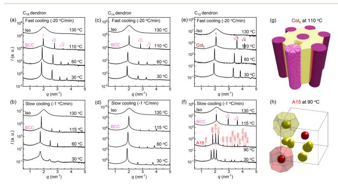
Fig. 2 SAXS intensity profiles of (a and b)  $C_{18}$ , (c and d)  $C_{14}$ , and (e and f)  $C_{12}$  dendrons with two different cooling rates of -20 and -1 °C min<sup>-1</sup> from 130 to 30 °C. 3D morphologies reproduced from the ED maps of (g) the stacked Col<sub>h</sub> and (h) A15 phases, which are obtained from the fast and slow cooling of the  $C_{12}$  dendrons, respectively.
