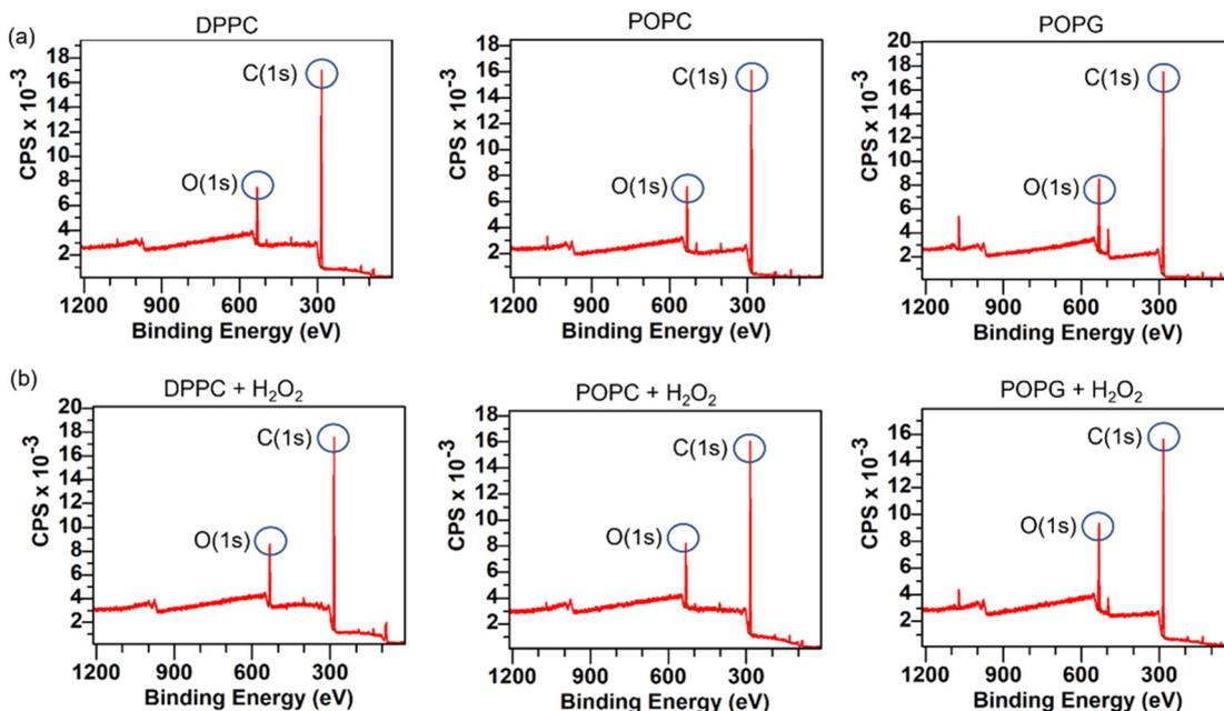
**Fig. 11** XPS spectra for the membranes before and after H<sub>2</sub>O<sub>2</sub>. The row (a) on top shows the spectra for the samples before being exposed to the oxidizing agent, while the row (b) on bottom displays the spectra from the same sample after being exposed to H<sub>2</sub>O<sub>2</sub>.
