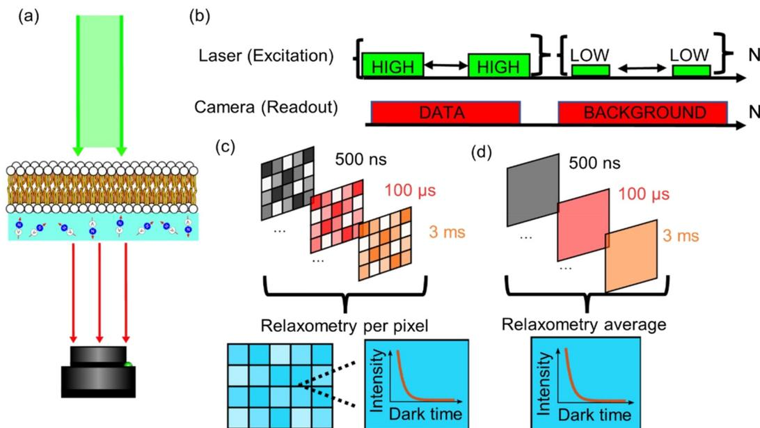
**Fig. 4** Experimental procedure. (a) Optical readout of the NV center and membrane system (simplified). (b) Pulsed sequence used in order to retrieve the  $T_1$  relaxometry information. (c) Grouping of the images for the relaxometry imaging procedure, in which every pixel contains a relaxometry curve. (d) Grouping of the images for the lipid peroxidation detection. In this case, all the pixels are added together to retrieve a single relaxometry curve.
