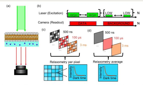
Fig. 4 Experimental procedure. (a) Optical readout of the NV center and membrane system (simplified). (b) Pulsed sequence used in order to retrieve the  $T_1$  relaxometry information. (c) Grouping of the images for the relaxometry imaging procedure, in which every pixel contains a relaxometry curve. (d) Grouping of the images for the lipid peroxidation detection. In this case, all the pixels are added together to retrieve a single relaxometry curve.
