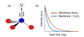
**Fig. 1** Diamond quantum relaxometry. (a) Physical structure of the nitrogen-vacancy (NV) center in diamond (b)  $\mathcal{T}_1$  relaxometry curve with and without the presence of paramagnetic species (in this case radical intermediates from lipid peroxidation).
