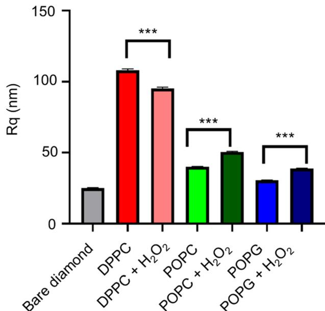
**Fig. 10** Analysis of the roughness of the AFM images. Statistical significance ( $N = 5$ ) was assessed with an unpaired  $t$ -test, having found statistical significance with all pairs. The bare diamond sample has a  $p < 0.001$  (\*\*\*\*) significant difference with all the pairs.
