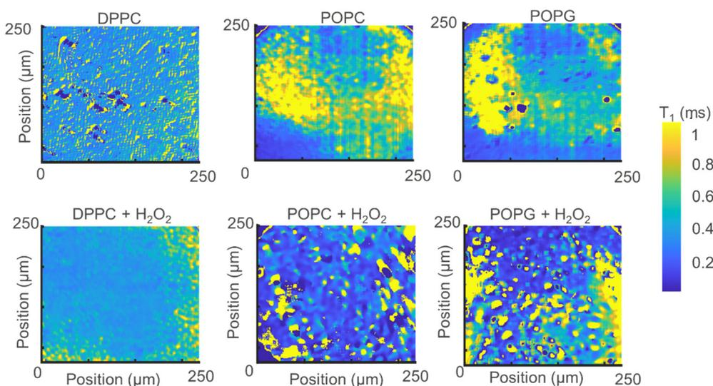
**Fig. 7** Relaxometry images of the different membranes (up) and the same membranes after exposure to H<sub>2</sub>O<sub>2</sub> (bottom).
