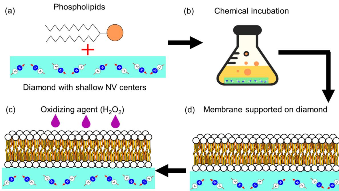
**Fig. 2** Overview of the planar lipid bilayer preparation and oxidation experiment. (a) Lipid structure and diamond sample with NV centres near the surface (b) Chemical incubation step. The lipid bilayer is grown right on top of the diamond sensor (c) Final structure. The lipid bilayer is supported in the diamond sensor (d) An oxidizing agent is added in order to initiate the lipid peroxidation process.
