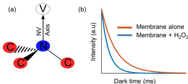
**Fig. 1** Diamond quantum relaxometry. (a) Physical structure of the nitrogen-vacancy (NV) center in diamond (b)  $T_1$  relaxometry curve with and without the presence of paramagnetic species (in this case radical intermediates from lipid peroxidation).
