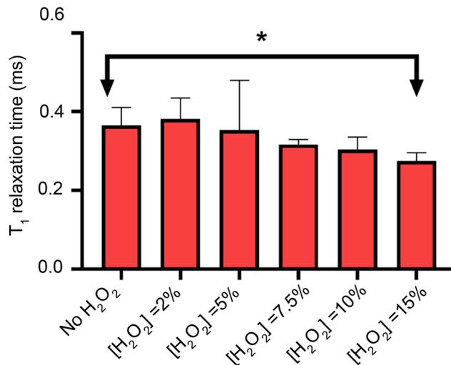
**Fig. 5** Effect of the hydrogen peroxide in the longitudinal relaxation time as a function of the oxidizing agent concentration. Each experiment shows the  $T_1$  relaxation time at different  $\text{H}_2\text{O}_2$  concentrations, including without  $\text{H}_2\text{O}_2$  (first experiment). Statistical significance ( $N = 6$ ) was assessed with an unpaired  $t$ -test, showing statistical significant differences only at 15% concentration v/v.
