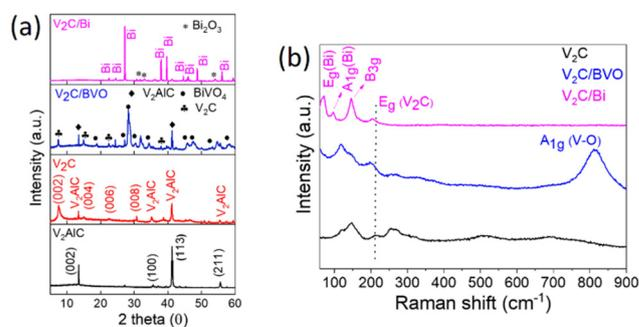
**Fig. 1** (a) XRD patterns of  $\text{V}_2\text{AlC}$ ,  $\text{V}_2\text{C}$ ,  $\text{V}_2\text{C}/\text{BVO}$ , and  $\text{V}_2\text{C}/\text{Bi}$ . (b) Raman spectra of  $\text{V}_2\text{C}$ ,  $\text{V}_2\text{C}/\text{BVO}$ , and  $\text{V}_2\text{C}/\text{Bi}$ .
