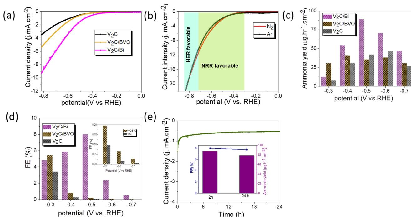
**Fig. 5** (a) Comparison of LSV curves of GC electrode,  $V_2C$ ,  $V_2C/BVO$ , and  $V_2C/Bi$  in  $N_2$ -saturated 0.1 M KOH with a scan rate of  $10$  mV s<sup>-1</sup>, (b) LSV curves of  $V_2C/Bi$  in Ar/ $N_2$ -saturated KOH electrolyte with a scan rate of  $10$  mV s<sup>-1</sup>, (c) corresponding  $NH_3$  yields (d) corresponding FE, (e) chronoamperometric test of  $V_2C/Bi$  at  $-0.5$  V for 24 h (insert: corresponding  $NH_3$  yields and FE after stability test).
