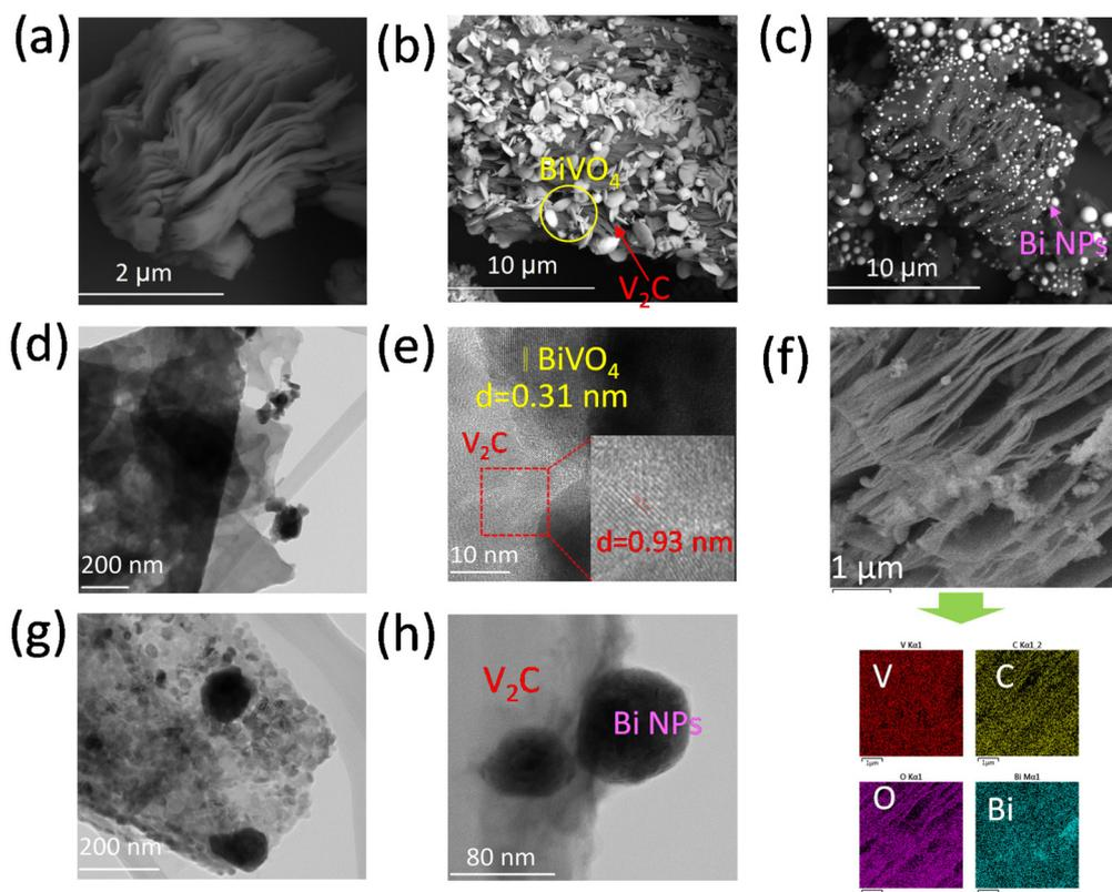
**Fig. 2** SEM of (a) V<sub>2</sub>C, (b) V<sub>2</sub>C/BVO and (c) V<sub>2</sub>C/Bi, (d) TEM of V<sub>2</sub>C/BVO, (e) HRTEM of V<sub>2</sub>C/BVO, (f) the main elemental components mapping of V, C, O and Bi of V<sub>2</sub>C/BVO, (g) TEM of V<sub>2</sub>C/Bi and (h) HRTEM of V<sub>2</sub>C/Bi.
