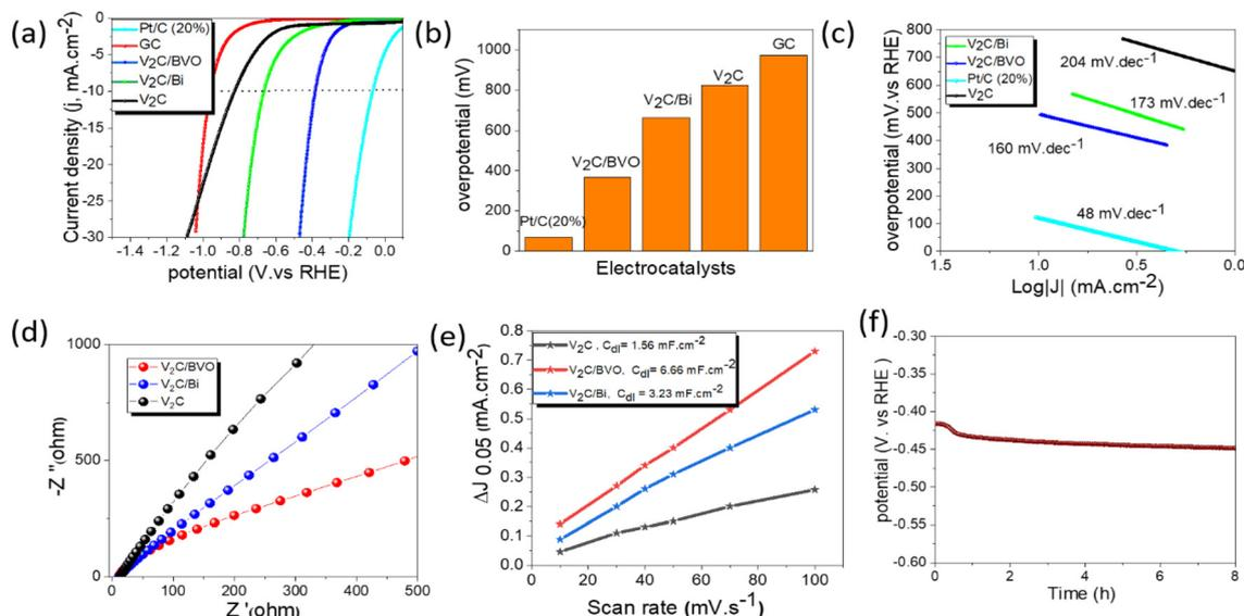
Fig. 4 Electrochemical measurements for hydrogen evolution in 0.5 M  $H_2SO_4$  acidic medium: (a) LSV curves, (b) onset overpotential at  $j = 10 \text{ mA cm}^{-2}$  of different electrocatalysts, (c) the corresponding Tafel plots, (d) EIS Nyquist plot of different catalysts, (e) capacitive  $\Delta j$  as a function of scan rates for different samples, and (f) the chronoamperometric measurement for  $V_2C/BVO$  at a constant current density of  $-10 \text{ mA cm}^{-2}$ .
