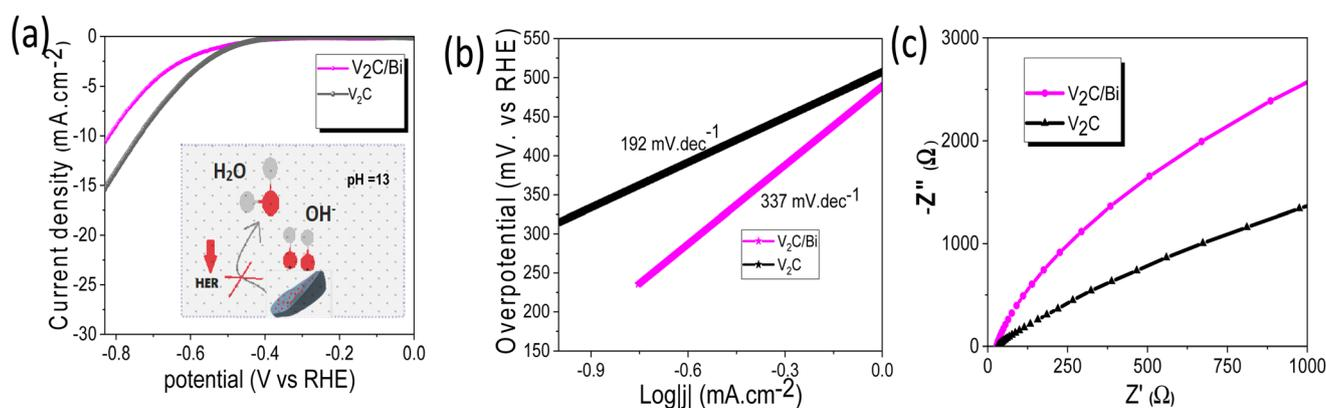
**Fig. 6** (a) LSV of  $V_2C/Bi$  and  $V_2C$  in Ar saturated KOH (insert: the deactivation mechanism of the HER process over  $V_2C/Bi$ ), (b) the corresponding Tafel plots analysis, and (c) EIS of  $V_2C$  and  $V_2C/Bi$ .
