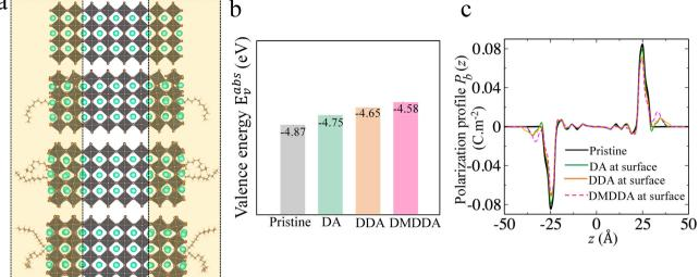
Fig. 4 (a) CsPbBr<sub>3</sub> CsBr terminated slabs without (top) and with DA, DDA and DMDDA ligands on the surface for a coverage of 11%. Corresponding (b) valence energies and (c) polarization density profiles.
