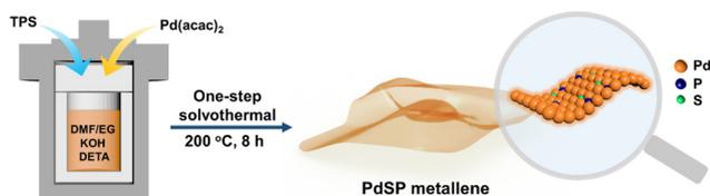
Fig. 1 Scheme for the preparation of PdSP metallene.
