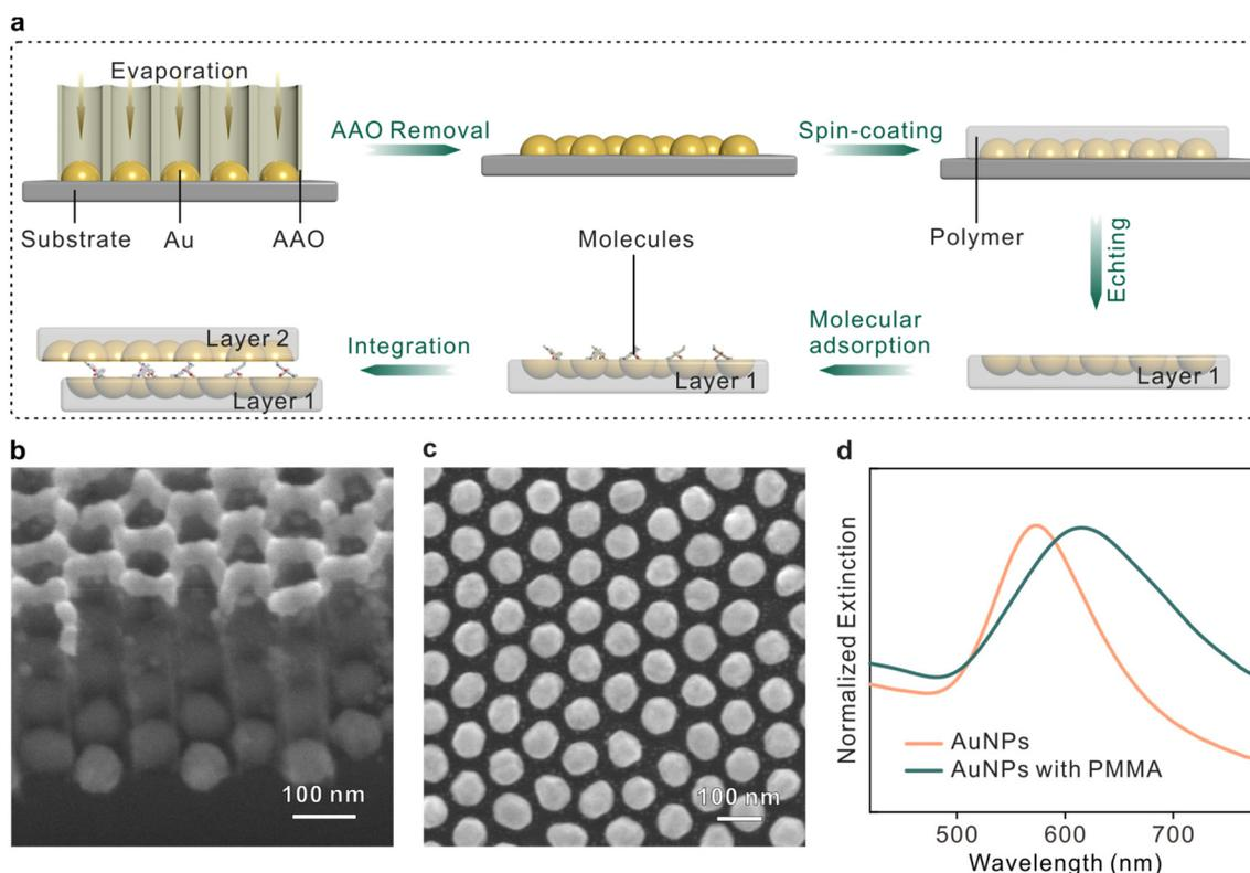
**Fig. 1** (a) Schematics illustrating the fabrication procedures of the sandwich plasmonic nanocavity. (b) Side view SEM image of the AuNPs with an AAO mask on silicon substrates. (c) Top view SEM image of the patterned AuNPs. (d) UV-vis spectra of the AuNPs with and without PMMA coating.
