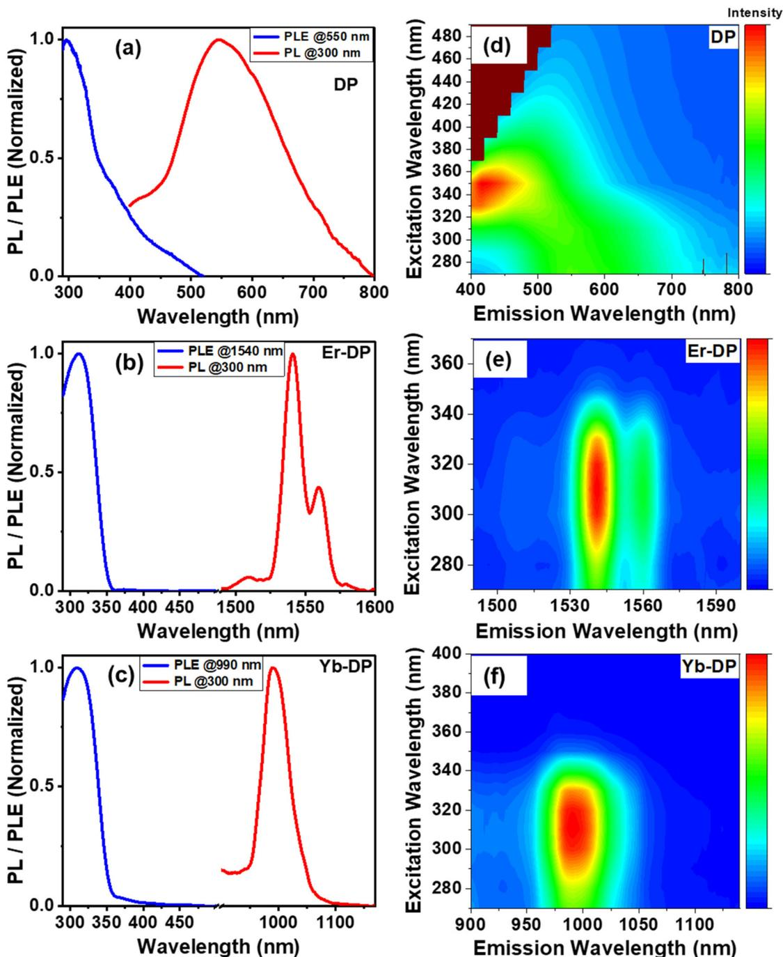
**Fig. 3** Photoluminescence (PL) curves at an excitation wavelength of 300 nm of (a) DP, (b) Er-DP and (c) Yb-DP. Photoluminescence excitation (PLE) curves at an emission wavelength of 550 nm for (a) DP, at an emission wavelength of 1450 nm for (b) Er-DP, and at an emission wavelength of 550 nm for (c) Yb-DP. Pseudo color plot between the excitation wavelength vs the emission wavelength at room temperature for (d) DP, (e) Er-DP and (f) Yb-DP.
