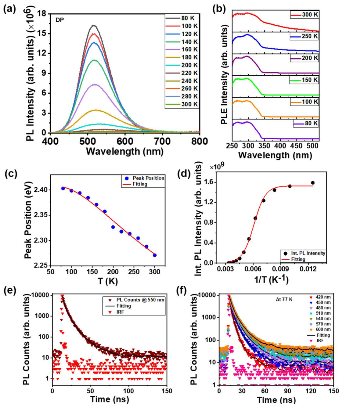
**Fig. 4** Temperature-dependent (a) PL at an excitation wavelength of 300 nm, (b) PLE at an emission wavelength of 550 nm, (c) PL peak position and (d) integrated PL intensity. (c) and (d) are associated with (a). (e) Room temperature time-resolved PL (TRPL) at an emission wavelength of 550 nm measured by TCSPC; (f) wavelength-dependent TRPL at 77 K. All the figures are for DP. Open scattered symbols represent experimental data and solid lines show theoretical fittings.
