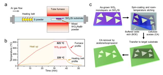
Fig. 1 Synthesis and transfer of  $WS_2$  monolayers for preparing  $WS_2/Ge$  heterostructures. (a) Schematic of the APCVD setup for synthesizing  $WS_2$  monolayers on  $SiO_2/Si$ . (b) Furnace and heating belt temperature profiles during the synthesis process. (c) Step-by-step schematics of the wet-transfer of  $WS_2$  onto target substrates using a cellulose acetate-assisted approach.
