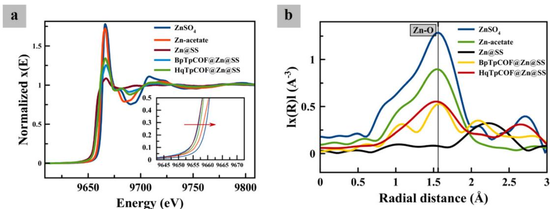
Fig. 3 (a) Zn K-edge XANES spectra at the surface of different zinc electrodes and (b) EXAFS spectra in the *R*-space for different zinc electrodes at  $1 \text{ mA h cm}^{-2}$  charged in a symmetrical cell.
