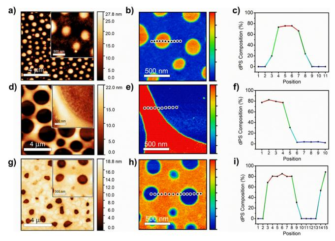
Fig. 2 Detailed height image, infrared image, and composition curve of (a-c) dPS: P3HT (1:3), (d-f) dPS: P3HT (1:1), and (q-i) dPS: P3HT (3:1).
