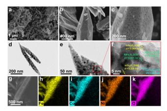
Fig. 1 (a-c) SEM images of Fe<sub>7</sub>Co<sub>1.5</sub>Ni<sub>1.5</sub> at different magnifications. (df) TEM and HR-TEM images of Fe<sub>7</sub>Co<sub>1.5</sub>Ni<sub>1.5</sub>. (g) EDS mapping images of (h) Fe, (i) Co, (j) Ni, and (k) O elements distributed at Fe<sub>7</sub>Co<sub>1.5</sub>Ni<sub>1.5</sub>.
