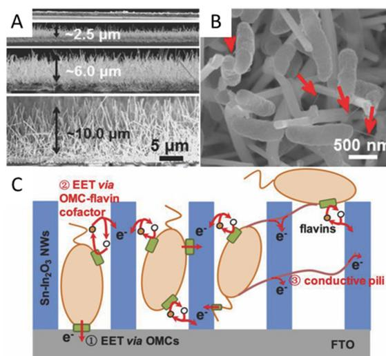
**Fig. 3** (A) Cross-section SEM images of the flat FTO film and SINW/FTO with the nanowire lengths of 2.47, 5.80, and 9.85  $\mu\text{m}$ . (B) SEM images of SINW/FTO electrodes integrated with microbes of *S. loihica* PV-4 after 25 h electrochemical culture at 0.2 V. The red arrows mark the pili grown among cells. (C) Cartoon illustrating the active EET pathways on the SINW/FTO electrode. Reproduced from ref. 133 with permission from Wiley Online Library, Copyright 2018.
