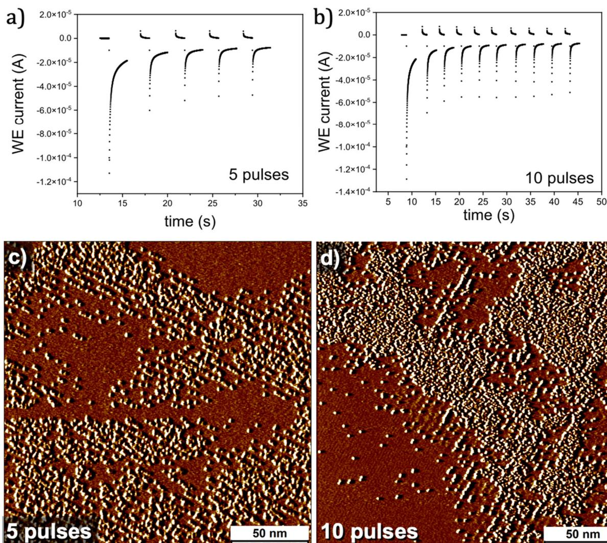
**Fig. 5** CV carried out using short potential pulses. Pulse potential:  $-0.35$  V, pulse width: 2 seconds, pulse interval: 0.5 seconds. Current profiles for (a) 5 pulses. (b) 10 pulses. (c and d) Representative STM images showing DMTC templated chemical patterning obtained using 5 and 10 potential pulses, respectively. Imaging parameters:  $V_{\text{bias}} = -0.9$  V,  $I_{\text{set}} = 0.05$  nA.
