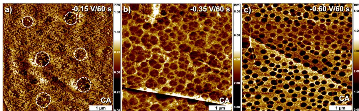
**Fig. 4** Tapping mode AFM topography images of covalently patterned graphite prepared using the DMTC template. The samples were prepared at (a)  $-0.15$  V; (b)  $-0.35$  V and (c)  $-0.60$  V. The electrolysis time was kept at 60 s for all samples. The white dashed circles in (a) highlight the areas with lower surface coverage of the organic film. For phase images see Fig. S10 in the ESI.†
