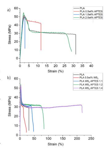
Fig. 9 Representative stress—strain curves for neat PLA relative to those for (a) blends of PLA and APTES and (b) composites of PLA and APTES modified WS $_2$  NTs.
