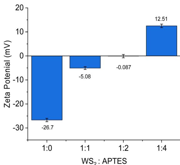
Fig. 6 ζ potential for WS<sub>2</sub> NTs, and change in ζ for APTES–WS<sub>2</sub> NTs with increasing APTES content.
