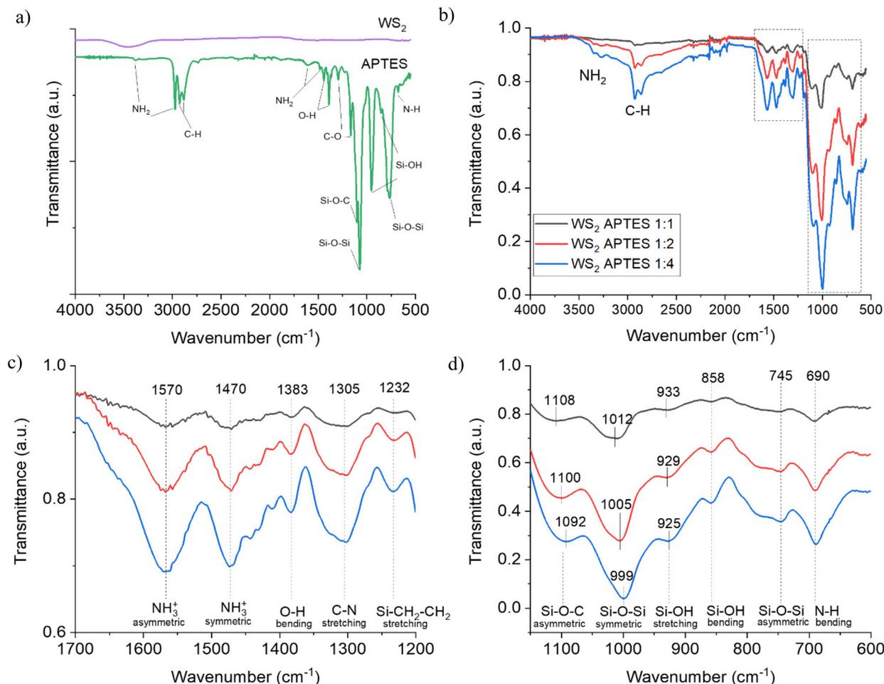
**Fig. 1** FTIR transmittance spectra of, (a) WS<sub>2</sub> NTs and APTES, (b) APTES functionalized WS<sub>2</sub> NTs in ratios of 1 : 1, 1 : 2 and 1 : 4, (c) spectra enlarged in the range 1700–1200 cm<sup>-1</sup> and (d) in the range 1150–600 cm<sup>-1</sup>.
