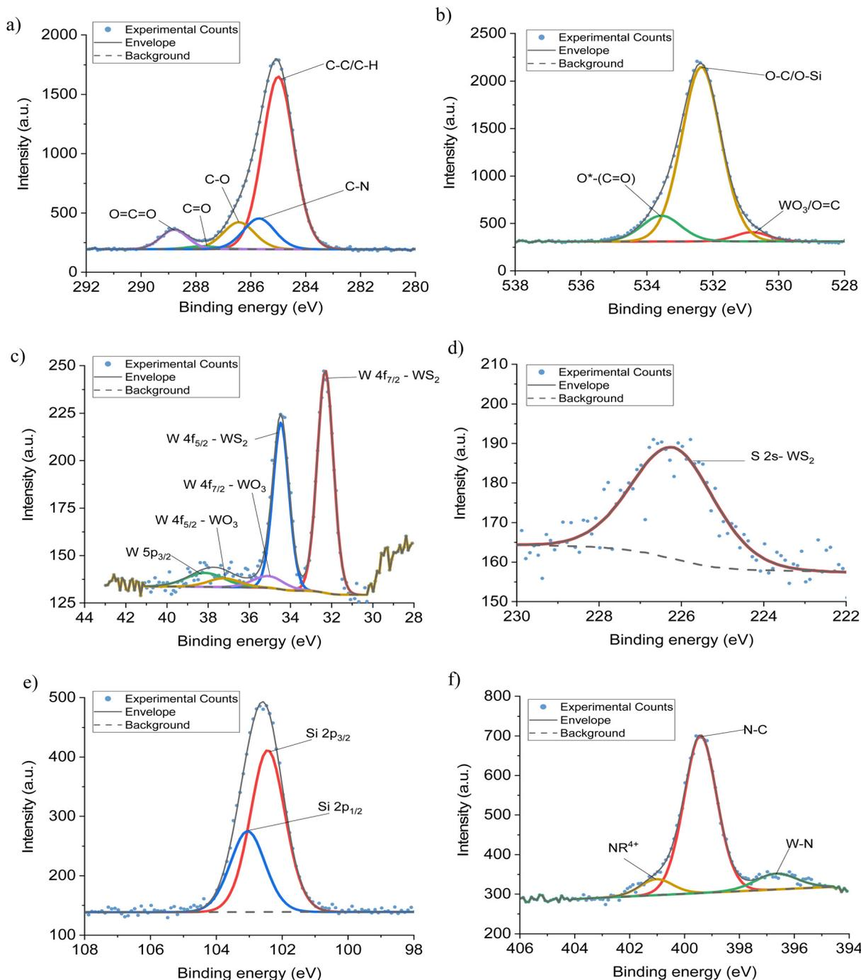
**Fig. 4** Deconvoluted XPS spectra, (a) C 1s, (b) O 1s, (c) W 4f, (d) S 2s, (e) Si 2p (f) N 1s regions from the XPS spectra of WS<sub>2</sub>-APTES at a ratio of 1 : 4.
