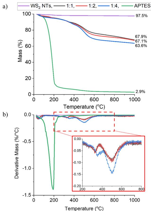
Fig. 2 (a) TGA weight loss curves and (b) DTA curves for WS<sub>2</sub> NTs, APTES and APTES modified WS<sub>2</sub> NTs at different ratios.
