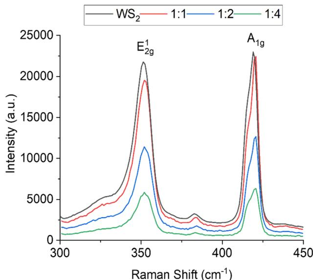
Fig. 3 Raman spectra of WS<sub>2</sub> NTs and APTES modified WS<sub>2</sub> NTs.
