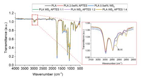
Fig. 7 FTIR spertra of for PLA, a blend of PLA and APTES composites of PLA with APTES modified WS2 NTs.
