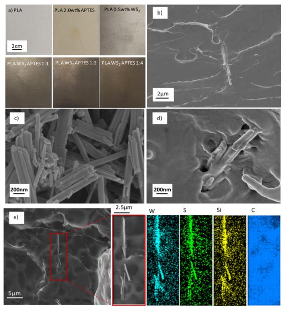
Fig. 8 (a) Representative optical photographs of film samples of PLA alone and corresponding composites and SEM micrographs of (b) composite of PLA and APTES modified WS2 NTs (1:4), (c) unmodified WS2 NTs, (d) composite of PLA and WS2 NTs: APTES 1:4 at higher magnification and (e) composite of PLA WS<sub>2</sub> NTs: APTES 1: 4 with corresponding EDS of highlighted area.
