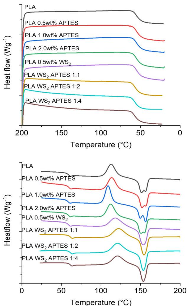
**Fig. 10** DSC thermograms for PLA and its blends with APTES and composites with APTES modified WS<sub>2</sub> NTs showing (a) first cooling cycle and (b) second heating cycle.
