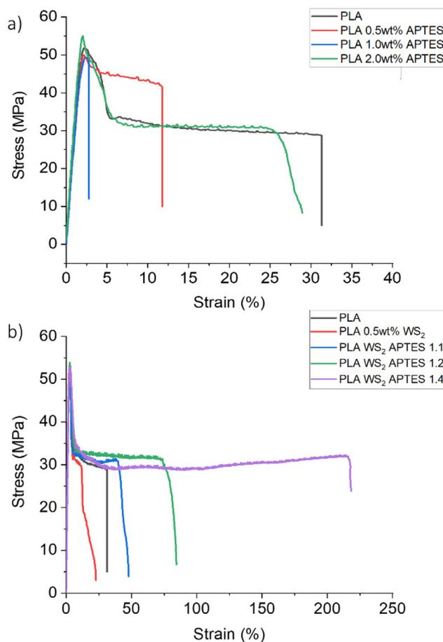
Fig. 9 Representative stress–strain curves for neat PLA relative to those for (a) blends of PLA and APTES and (b) composites of PLA and APTES modified WS<sub>2</sub> NTs.
