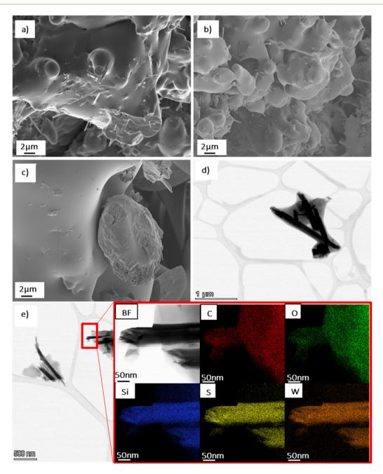
Fig. 5 SEM and STEM imaging of APTES functionalised WS<sub>2</sub> NTs. (a-c) SEM images of WS<sub>2</sub> NTs: APTES at 1:1, 1:2 and 1:4, respectively. (d) STEM of WS2 NTs: APTES at 1:4, and (e) STEM and EDS mapping of the WS2NTs-APTES 1:4 sample.
