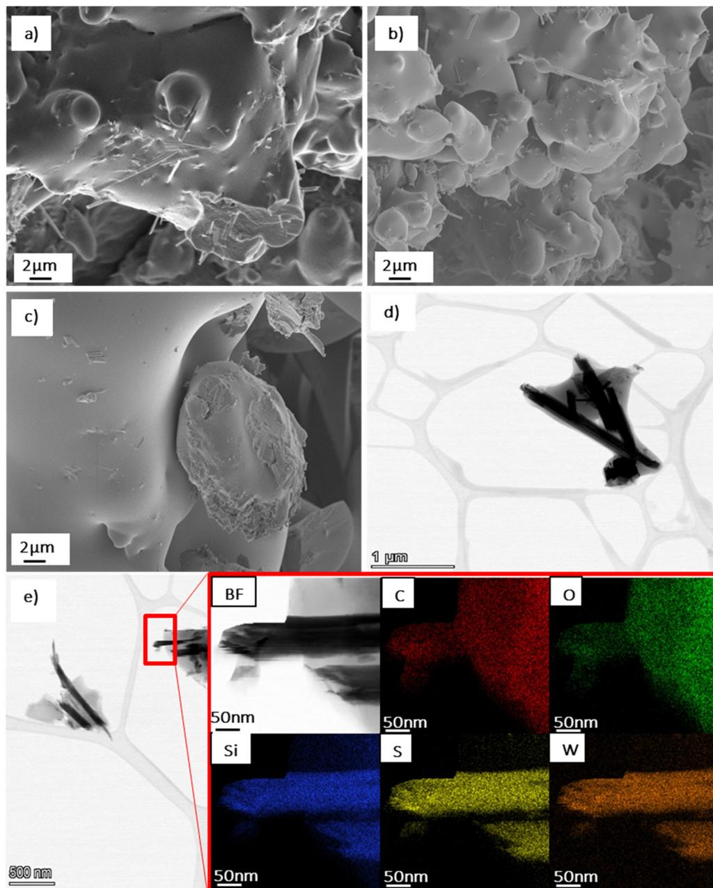
**Fig. 5** SEM and STEM imaging of APTES functionalised WS<sub>2</sub> NTs. (a–c) SEM images of WS<sub>2</sub> NTs : APTES at 1 : 1, 1 : 2 and 1 : 4, respectively. (d) STEM of WS<sub>2</sub> NTs : APTES at 1 : 4, and (e) STEM and EDS mapping of the WS<sub>2</sub>NTs–APTES 1 : 4 sample.
