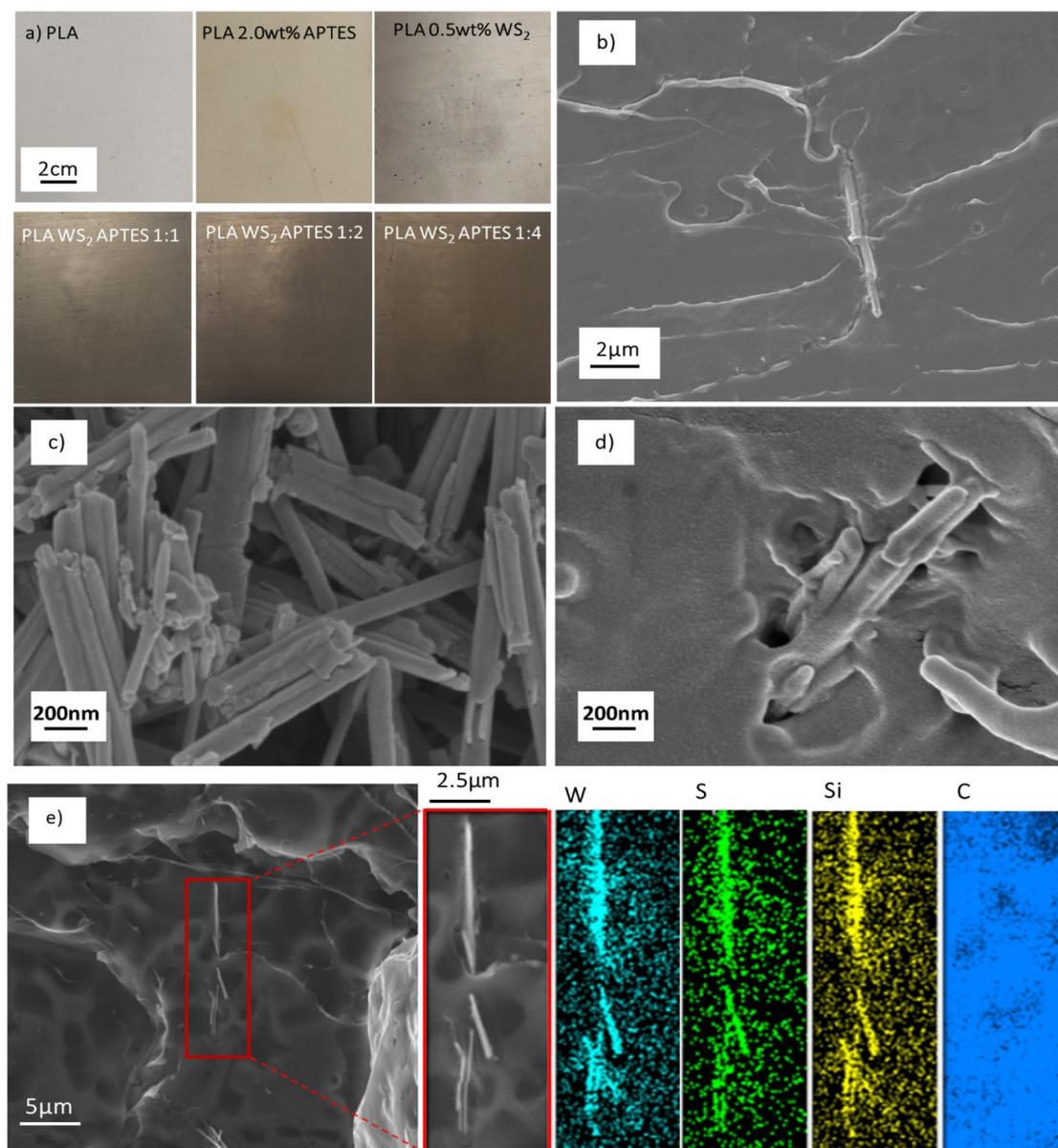
**Fig. 8** (a) Representative optical photographs of film samples of PLA alone and corresponding composites and SEM micrographs of (b) composite of PLA and APTES modified WS<sub>2</sub> NTs (1 : 4), (c) unmodified WS<sub>2</sub> NTs, (d) composite of PLA and WS<sub>2</sub> NTs : APTES 1 : 4 at higher magnification and (e) composite of PLA WS<sub>2</sub> NTs : APTES 1 : 4 with corresponding EDS of highlighted area.
