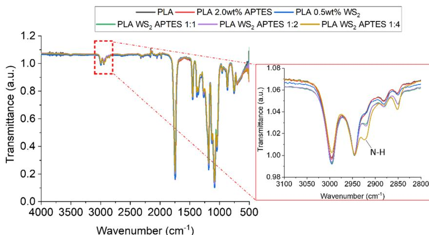
Fig. 7 FTIR spectra of PLA, a blend of PLA and APTES composites of PLA with APTES modified WS<sub>2</sub> NTs.
