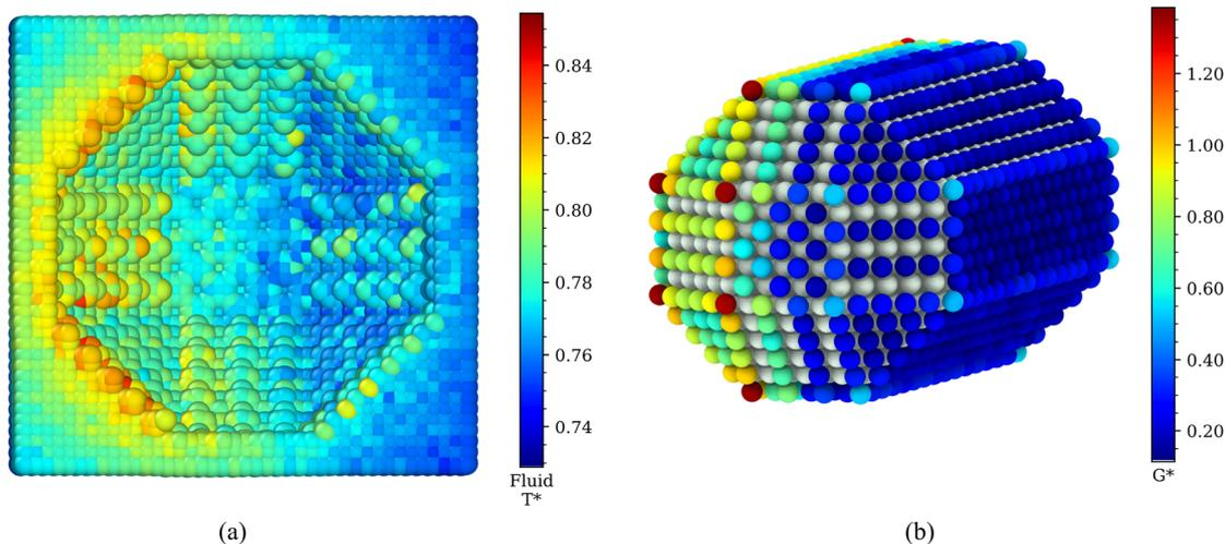
**Fig. 9** (a) Solvent temperature  $T^*$  around the Janus nanorod. (b) Interfacial thermal conductance  $G^*$ , projected on the Janus nanorod's surface atoms. The blue region corresponds to the lyophobic side of the nanorod.
