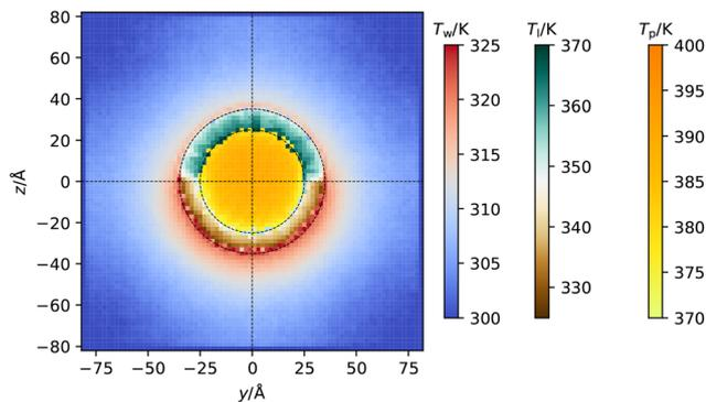
**Fig. 6** Spatially varying temperature in the  $y$ - $z$  plane (see Fig. 1 for information on the axes) in a slab of thickness 10 Å that cuts the centre of the nanoparticle. Three different colour scales are used to highlight the different temperature ranges covered by each component of the system, which from left to right are the temperature of the water ( $T_w$ ), ligands ( $T_l$ ) and gold core ( $T_p$ ).
