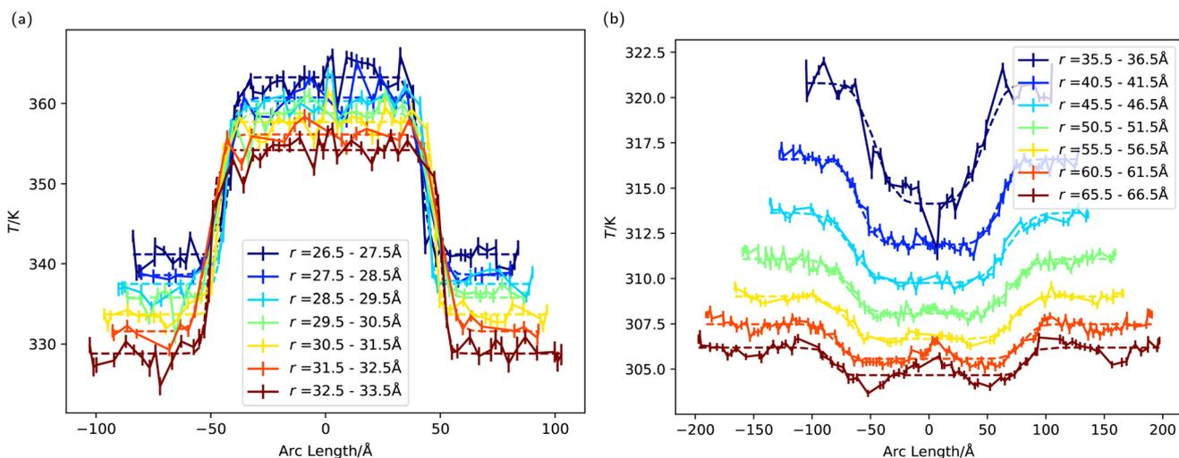
**Fig. 7** (a) The temperature of the ligands as a function of arc length, with an angle of zero corresponding to the direction parallel to the  $z$  axis. These temperature profiles were fitted to eqn (5) (see main text). (b) The water temperature as a function of arc length, with an angle of zero corresponding to the direction parallel to the  $z$  axis.
