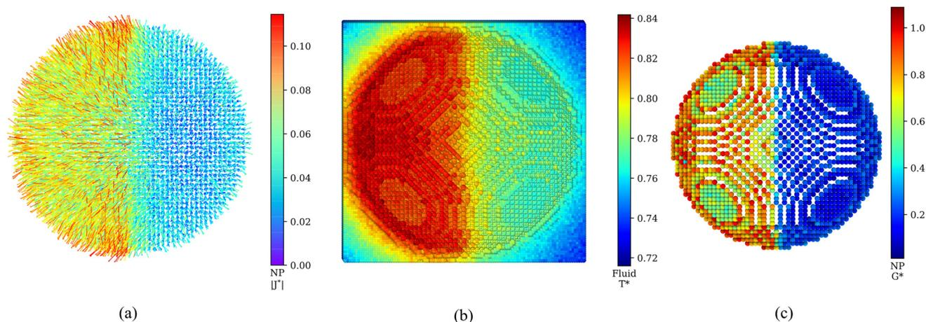
**Fig. 3** (a) Local Heat flux at the NP surface projected on the surface atoms. The arrows represent the local direction and magnitude of the heat fluxes. (b) Radial temperature ( $T^*$ ) profiles of the fluid (solvent) in contact with the lyophilic ( $F = 0.25$ ) or lyophobic ( $F = 0.10$ ) side of the Janus nanoparticle. (c) Local Interfacial Kapitza conductance projected on the surface atoms.
