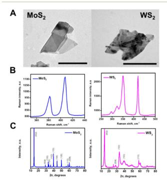
Fig. 2 Characterization of the microflakes. (A) TEM images of the MoS<sub>2</sub> and WS2 microflakes. (B) Raman spectra of each microflake and (C) XRD patterns of both materials. Scale bars, 500 nm.
