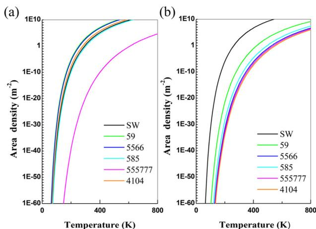
**Fig. 2** The areal density of various defects *versus* temperature for (a)  $\alpha$ -antimonene and (b) phosphorene. The defects considered include SW, SV-(5|9), SV-(55|66), DV-(5|8|5), DV-(555|777) and DV-(4|10|4).
