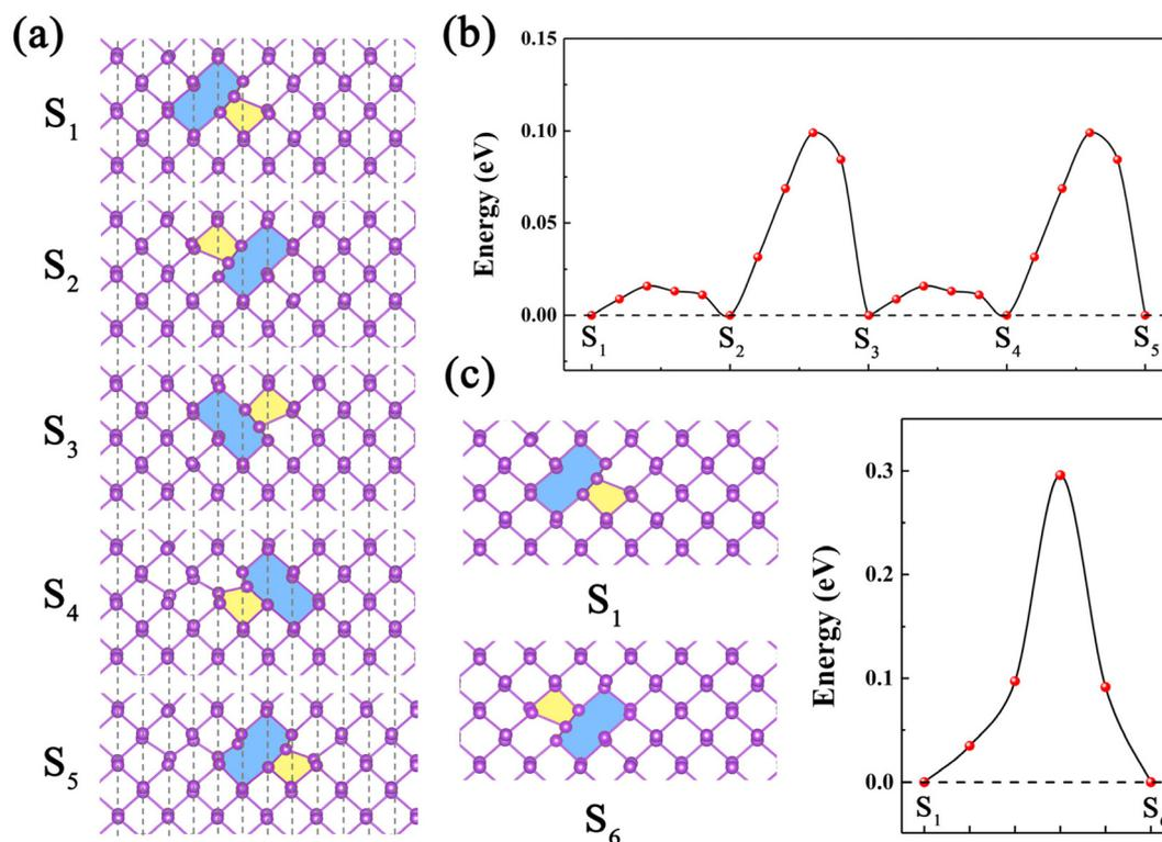
**Fig. 3** (a) Intermediates states ( $S_1$ – $S_5$ ) for the SV-(5|9) defect diffusion along the zigzag direction between neighboring equivalent sites. (b) Energetic profiles for the diffusion of the vacancy from  $S_1$  to  $S_5$ . (c) Computed energy barrier for interchain vacancy diffusion from  $S_1$  to  $S_6$ .
