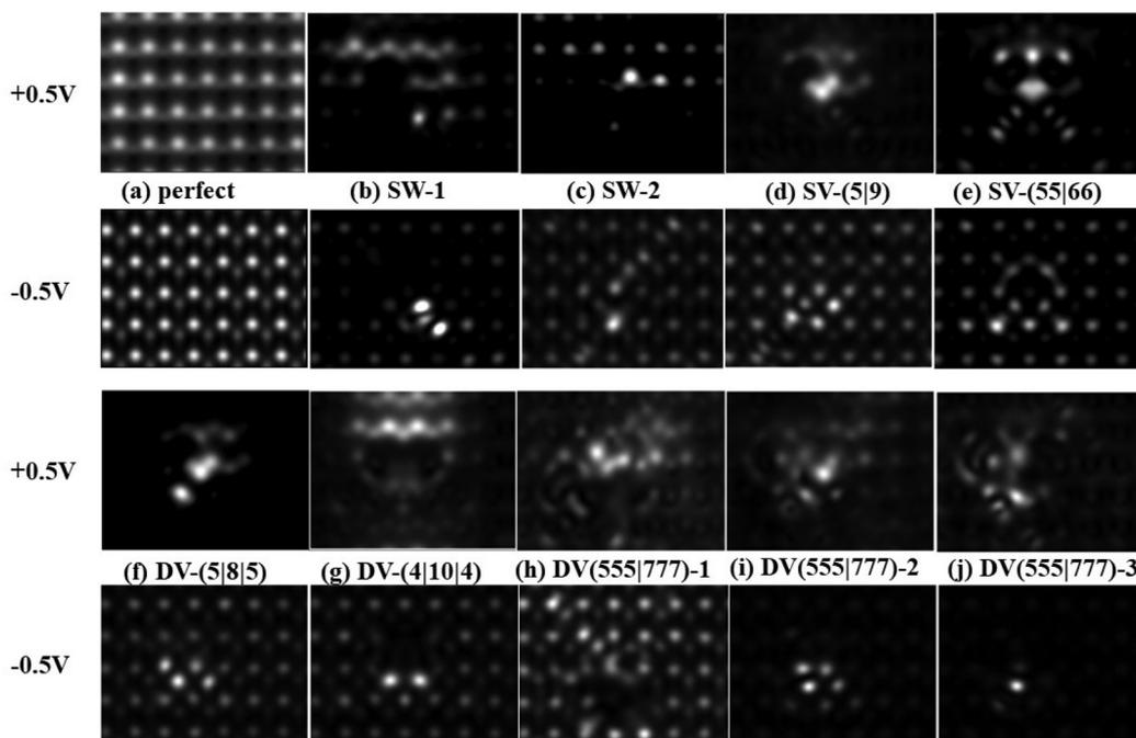
**Fig. 6** Simulated STM image of the perfect  $\alpha$ -antimonene (a) and defective  $\alpha$ -antimonene with defect: (b) SW-1; (c) SW-2; (d) SV-(5|9); (e) SV-(55|66); (f) DV-(5|8|5); (g) DV-(4|10|4); (h) DV(555|777)-1; (i) DV(555|777)-2; (j) the simulated STM image of DV-(555|777)-3 at a distance of 2 Å from the surface.
