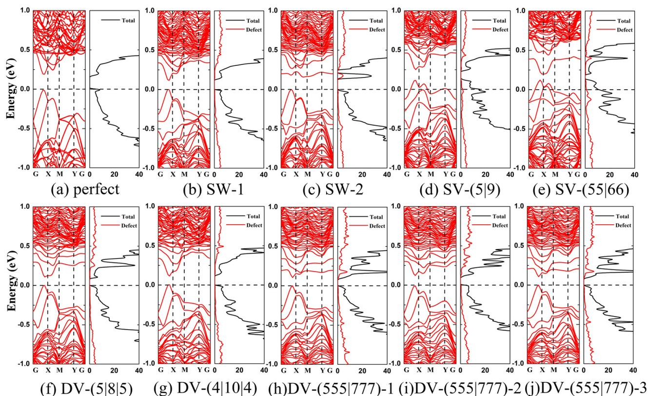
Fig. 4 Computed electronic band structure and density of states of various  $\alpha$ -antimonenes without or with defects: (a) perfect;  $\alpha$ -antimonene with defects of (b) SW-1; (c) SW-2; (d) SV-(5|9); (e) SV-(55|66); (f) DV-(5|8|5); (g) DV-(4|10|4); (h) DV-(555|777)-1; (i) DV-(555|777)-2; and (j) DV-(555|777)-3.
