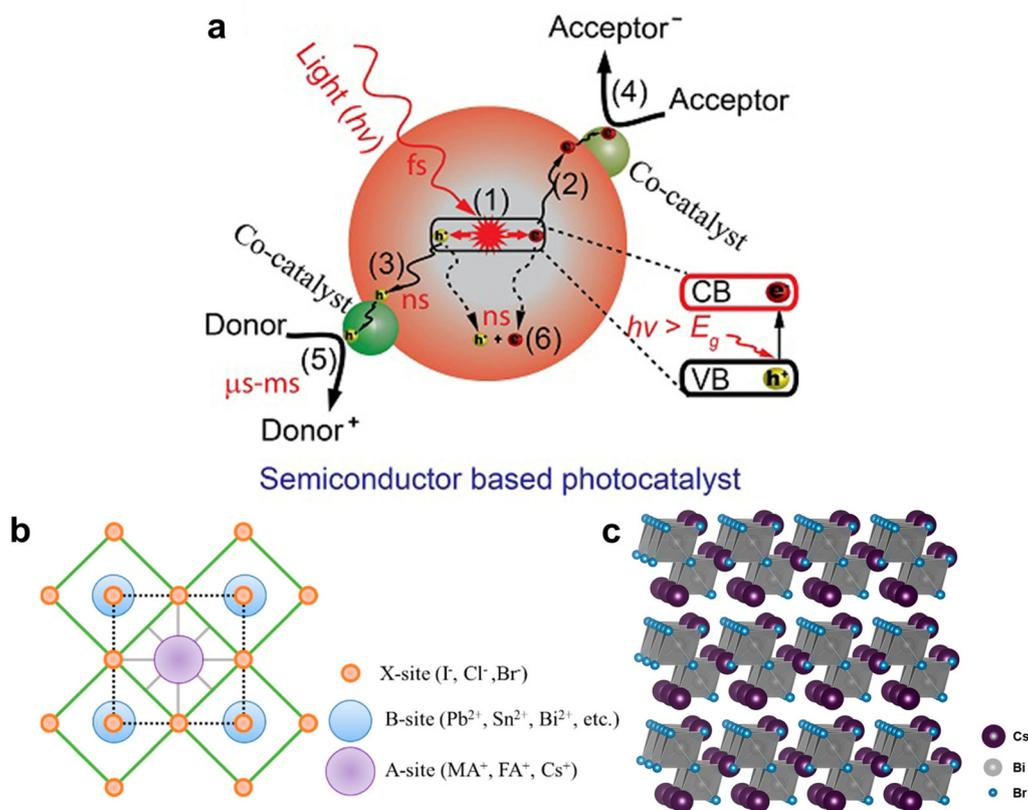
**Fig. 1** (a) Fundamental working principles of a semiconductor-based photocatalyst. Reproduced with permission from ref. 11. Copyright 2022 Tsinghua University Press. (b) The typical crystal structure of MHPs. Reproduced with permission from ref. 73. Copyright 2020 MDPI. (c) The typical crystal structure of  $Cs_3Bi_2Br_9$ . Reproduced with permission from ref. 77. Copyright 2016 American Chemical Society.
