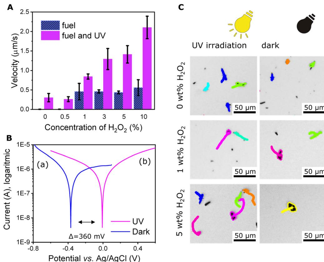
**Fig. 3** Characterization of the locomotion of the microrobots. (A) Average velocity of microrobots at different fuel concentrations and the influence of UV irradiation. (B) Tafel plots of static microrobots to demonstrate photocatalytic activity. The Tafel curves were measured in pure water under dark conditions (a) and under UV irradiation (b). (C) Typical trajectories of microrobots at different conditions collected after 20 s.
