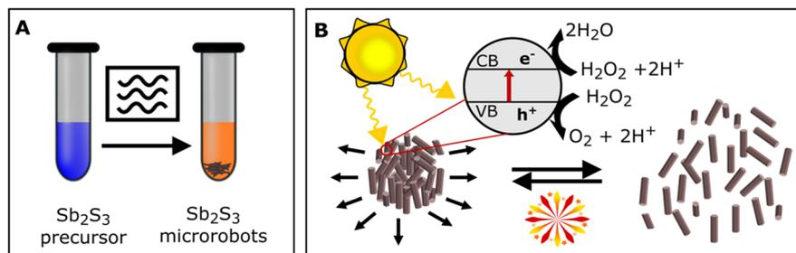
**Fig. 1** Schematic illustration showing (A) the “one-pot” preparation of  $\text{Sb}_2\text{S}_3$  microrobots using a microwave reactor and (B) their phoretic properties under light irradiation that induce swarming-like behavior. CB and VB stand for conduction and valence bands, respectively.
