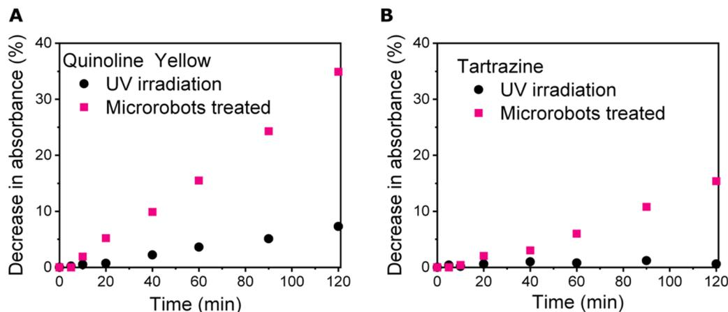
**Fig. 5** Photodegradation of food dyes determined by the change in absorbance. Graphs show degradation of quinoline yellow (A) and tartrazine (B) using photocatalytically active microrobots and UV irradiation alongside the control experiment where no microrobots were applied.
