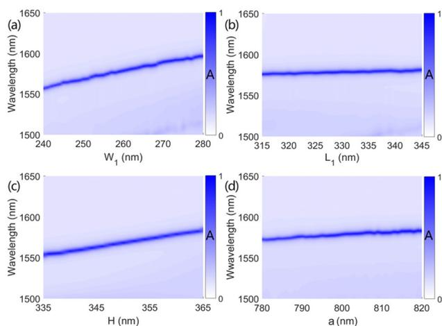
**Fig. 6** The dependence of absorptance spectra on structural parameters. Absorptance spectra as a function of  $W_1$  (a),  $L_1$  (b),  $H$  (c), and  $a$  (d), respectively. Other simulated details are identical to those used in Fig. 5(a), except the variable parameter in each subfigure.
