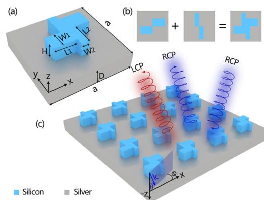
**Fig. 1** Schematic illustration of the designed chiral metasurface on a silver substrate. (a) Geometry of the unit cell. (b) The top view of the unit cell. (c) Illustration of the periodic planar metasurface illuminated by circularly polarized light with the incident angle  $\theta$  relative to  $z$  axis and the azimuthal angle  $\phi$  relative to  $x$  axis.
