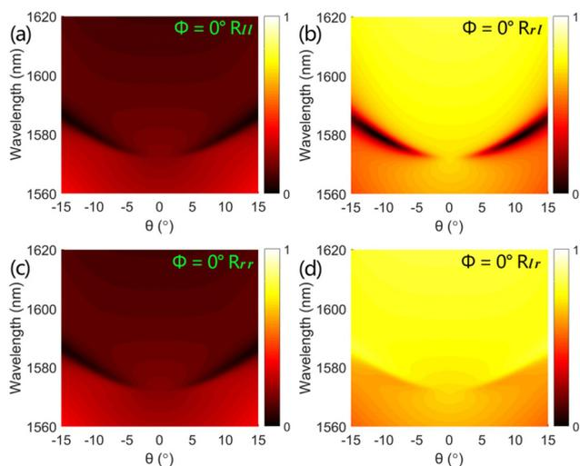
**Fig. 3** The evolution of reflection spectra of all Jones matrix elements on the incident angle  $\theta$  that varies along the  $x$  axis (*i.e.*, the azimuthal angle is  $\Phi = 0^\circ$ ). (a)–(d) correspond to the Jones matrix elements of  $R_{ll}$ ,  $R_{rl}$ ,  $R_{rr}$ , and  $R_{lr}$ , respectively.
