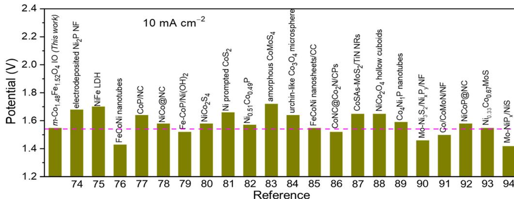
**Fig. 8** Comparison of the overall water splitting activity of m- $\text{Co}_{1.48}\text{Fe}_{1.52}\text{O}_4$  IO ( $1\text{Co1Fe}$  catalyst) with other non-noble metal-based electrocatalysts in alkaline electrolytes.
