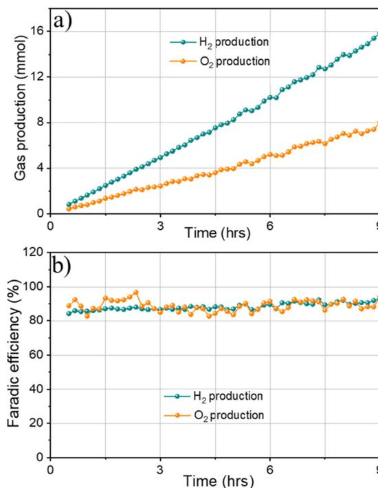
**Fig. 9** (a) Amounts of  $\text{H}_2$  and  $\text{O}_2$  gases and (b) faradaic efficiency obtained from  $1\text{Co1Fe}$  electrode-pair setting ( $\eta = 540 \text{ mV}$ ) by GC measurement versus time for electrolysis with a current density of  $100 \text{ mA cm}^{-2}$  in 1 M KOH aqueous solution.
