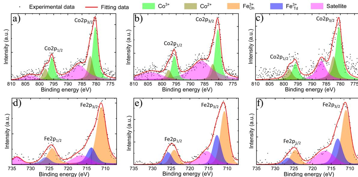
**Fig. 3** Co 2p (a, b and c) and Fe 2p (d, e and f) XPS spectra of 2Co1Fe (a and d), 1Co1Fe (b and e) and 1Co2Fe (c and f). The black points are the experimental data and the red lines are the corresponding fitting curves. The shaded areas underneath the fitting curves are Voigt functions, representing the individual contributions.
