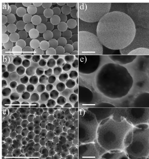
**Fig. 1** SEM images illustrating the different steps of the fabrication process of the 1Co1Fe mesoporous inverse opal structure: (a) PS beads as hard template, (b) the precursor solution-treated PS-coated substrates after drying and annealing at 200 °C for 3 h, (c) 1Co1Fe IO obtained after calcination at 500 °C for 2 h. Scale bars are 1  $\mu\text{m}$ . The respective high-resolution enlarged SEM images in the right column (d–f) have scale bars of 100 nm.
