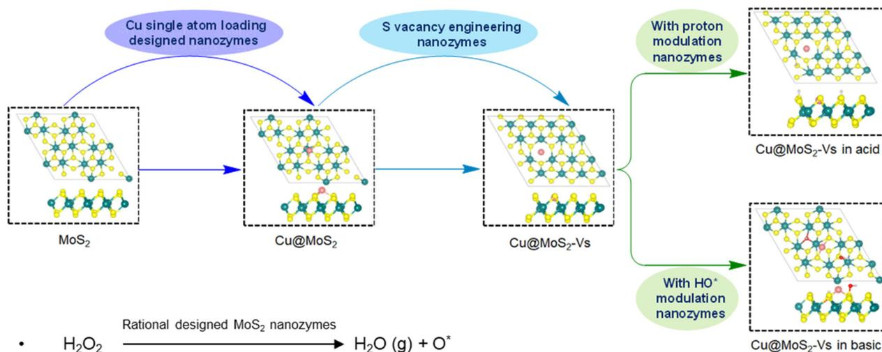
**Fig. 1** A schematic diagram of the rational design of MoS<sub>2</sub> nanozymes to modulate peroxidase-like activity through surface modification with Cu single atom loading, sulfur vacancy and acidic and alkaline environment regulation. The spheres in green, yellow, pink, red and gray represent Mo, S, Cu, O and H atoms, respectively.
