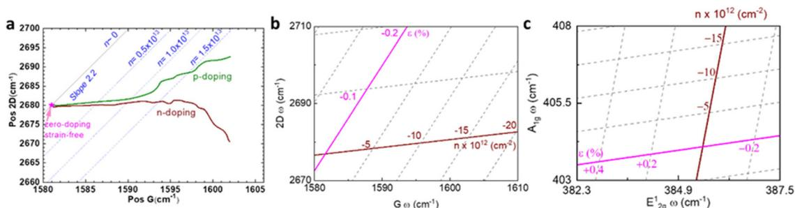
Fig. 7 Illustration of strain and doping correlation plot (Pos G vs. Pos 2D) of (a) graphene for both p- and n-doping, (b) graphene for only p-doping, and (c) MoS<sub>2</sub>. Each Raman dataset in G-2D axes represent the corresponding strain and doping in  $\epsilon$ - $n$  axes.
