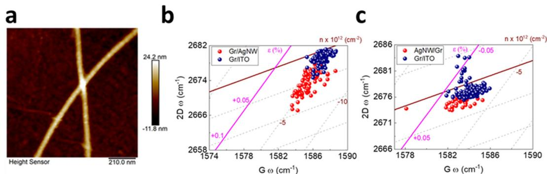
**Fig. 13** (a) AFM image of graphene covered AgNW. (b) Correlation plot of Gr/AgNW and (c) AgNW/Gr heterostructure. Blue colour represents bare graphene while red colour represents incorporation of AgNW. Reprinted with permission from ref. 5 Copyright (2022) from MDPI.
