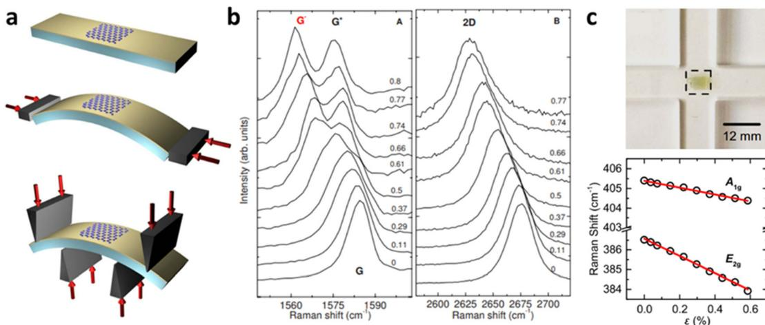
**Fig. 8** Determination of Grüneisen parameters: (a) Schematic diagram of bending of graphene on PET substrate and (b) the corresponding Raman shift with increasing tensile strain. Reprinted with permission from ref. 8 Copyright (2022) from American Physical Society. (c) Illustration of MoS<sub>2</sub> bending measurement and its influence on Raman shift. Reprinted with permission from ref. 22 Copyright (2022) from IOP Publishing.
