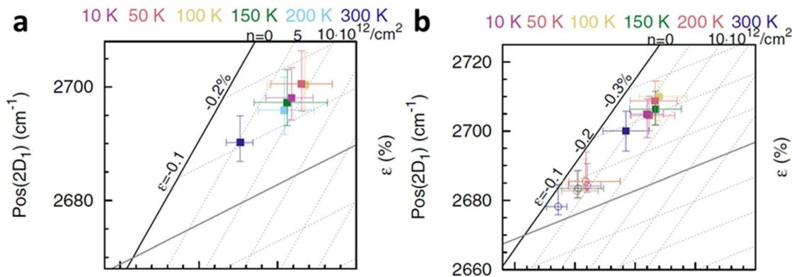
**Fig. 15** Temperature-dependent strain and doping of (a) monolayer graphene and (b) isotopically labelled bilayer graphene. Open circles represent the top layer while filled squares represent the bottom layer. Reprinted with permission from ref. 6 Copyright (2022) from American Physical Society.
