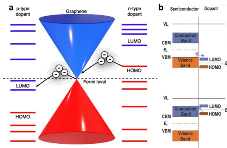
**Fig. 3** Charge transfer mechanism between 2D materials and surface dopant: (a) schematic diagram of the energy bands of graphene with different electron affinities of the dopant. Reprinted with permission from ref. 3 Copyright (2022) from Beilstein Journal of Nanotechnology. (b) Schematic band diagram of the semiconductor based 2D materials towards surface dopants. Reprinted with permission from ref. 17 Copyright (2022) from John Wiley and Sons.
