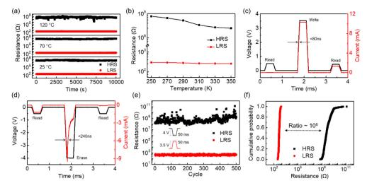
Fig. 3 (a) Retention performance of the memristor at 25 °C, 70 °C, and 120 °C. (b) The plot of resistances at HRS and LRS with the temperature. (c) The time-dependent current response of the C-h-BN memristor under pulsed write and read voltages. (d) The time-dependent current response of the C-h-BN memristor under pulsed erase and read voltages. (e) Endurance performance of the memristor. (f) Cumulative probability of the resistance at HRS and LRS.
