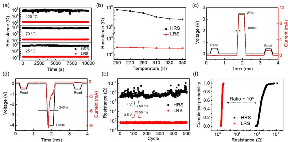
**Fig. 3** (a) Retention performance of the memristor at 25 °C, 70 °C, and 120 °C. (b) The plot of resistances at HRS and LRS with the temperature. (c) The time-dependent current response of the C-h-BN memristor under pulsed write and read voltages. (d) The time-dependent current response of the C-h-BN memristor under pulsed erase and read voltages. (e) Endurance performance of the memristor. (f) Cumulative probability of the resistance at HRS and LRS.
