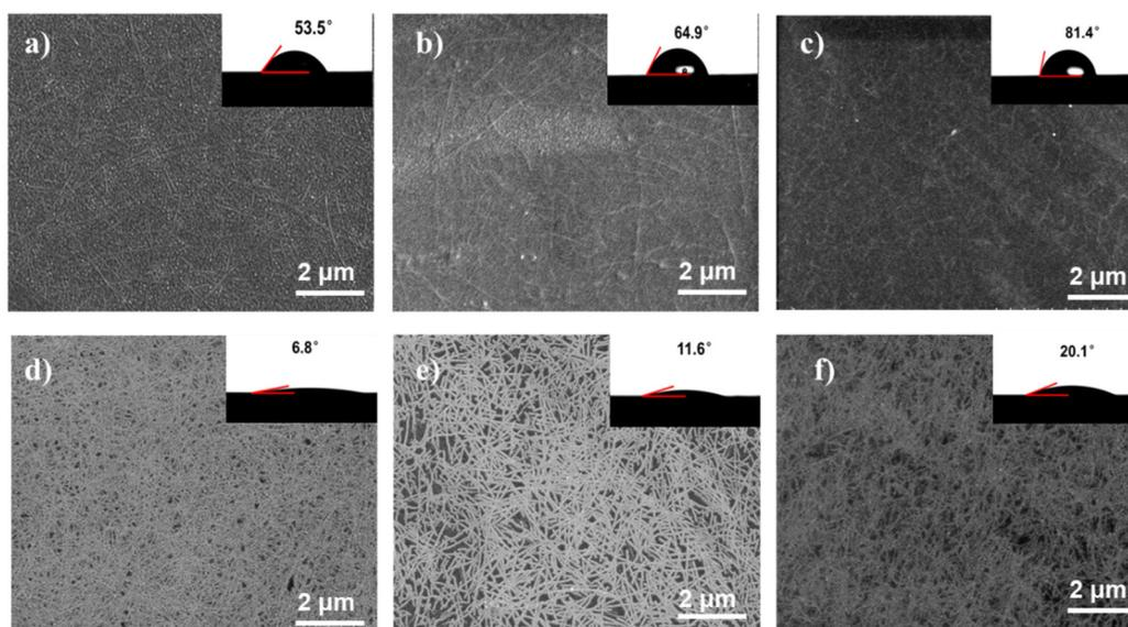
**Fig. 2** SEM images of sc-SWCNT films on (a) Al, (b) PET, and (c) paper substrates without the c-PVP modification layer, and (d) Al, (e) PET and (f) paper substrates with c-PVP modification after R2R printing 10 times. The insets are water contact angles of Al, PET, and paper substrates before and after the modification of c-PVP thin films by R2R gravure printing.
