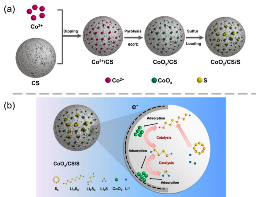
**Fig. 1** (a) Schematic diagram of synthesis process of CoO<sub>x</sub>/CS/S composites. (b) Schematic illustration of electrochemical reactions of the CoO<sub>x</sub>/CS cathode in the Li-S battery.
