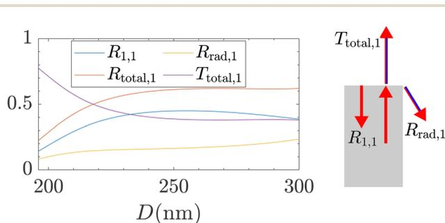
**Fig. 6** Reflection and transmission of the fundamental mode as a function of the diameter,  $D$ , at the top interface. A sketch of top interface and the reflection and transmission of the fundamental mode is seen to the right.
