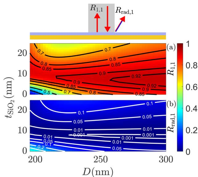
**Fig. 7** (a) Modal reflection,  $R_{1,1}$  and (b) reflection into radiation of the fundamental mode,  $R_{\text{rad},1}$ , as a function of the diameter,  $D$ , and silica layer thickness,  $t_{\text{SiO}_2}$ , at the bottom interface. A sketch of the bottom interface is shown in the top part of the figure.
