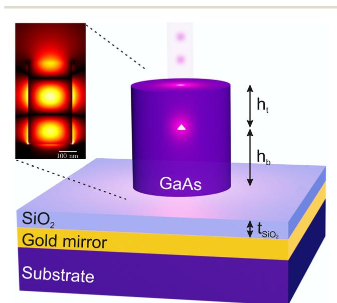
**Fig. 1** Sketch of the “nanopost” nanowire optical nanocavity and the geometrical parameters. The resulting in-plane electrical field profile of a QD placed inside the nanopost is shown as an inset. The length of the white scale bar in the inset is 100 nm.
