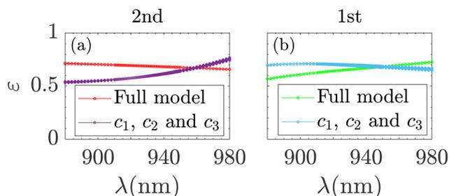
**Fig. 14** Efficiency,  $\varepsilon$  (NA = 0.75), as a function of the wavelength,  $\lambda$ , for the 2nd antinode (a) and 1st antinode (b). The full model is compared to only using  $c_1$ ,  $c_2$  and  $c_3$ .  $D = 238$  nm and  $t_{\text{SiO}_2} = 0$  nm. The thickness of the curves represents the numerical uncertainty.
