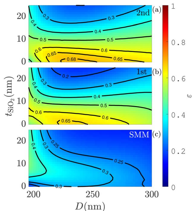
Fig. 3 Collection efficiency,  $\epsilon$  ( $\text{NA} = 0.75$ ), for a QD at the 2nd antinode (a), 1st antinode (b) and any antinode using the SMM (c) as a function of the diameter,  $D$ , and the silica layer thickness,  $t_{\text{SiO}_2}$ .
