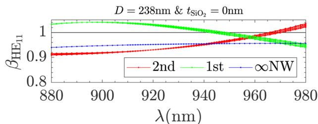
**Fig. 13**  $\beta_{\text{HE}_{11}} = P_{\text{HE}_{11}}/P_{\text{T}}$  as a function of the wavelength,  $\lambda$ , for the 2nd and 1st antinode and the infinite nanowire. The numerical uncertainty is represented by the thickness of the curves.
