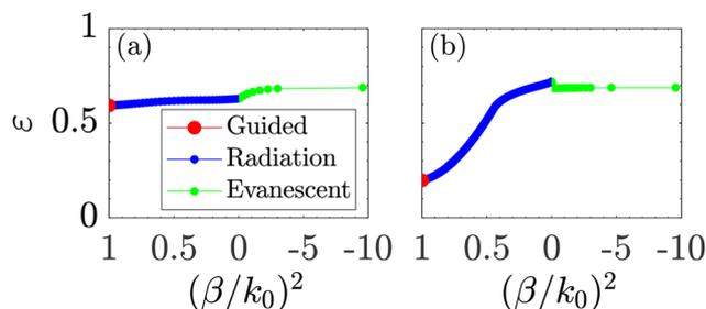
**Fig. 8** (a) Efficiency,  $\epsilon$  (NA = 0.75), as a function of the initial coefficients expressed with the propagation constant  $(\beta/k_0)^2$ . (b) Efficiency,  $\epsilon$  (NA = 75), as a function of the final coefficients expressed with the propagation constant  $(\beta/k_0)^2$ .
