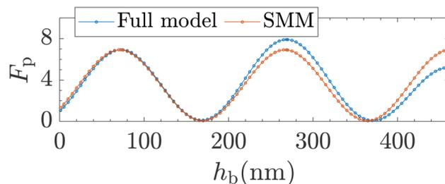
Fig. 10 Purcell factor,  $F_p$ , computed using the full model and SMM as a function of the dipole position from the bottom interface,  $h_b$ .  $D = 250$  nm and  $t_{\text{SiO}_2} = 13$  nm.
