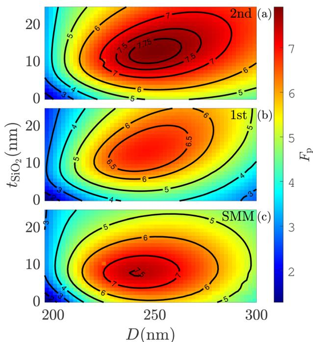
Fig. 2 Purcell factor,  $F_p$ , for a QD at the 2nd antinode (a), 1st antinode (b) and any antinode using the SMM (c) as a function of the diameter,  $D$ , and the silica layer thickness,  $t_{\text{SiO}_2}$ .
