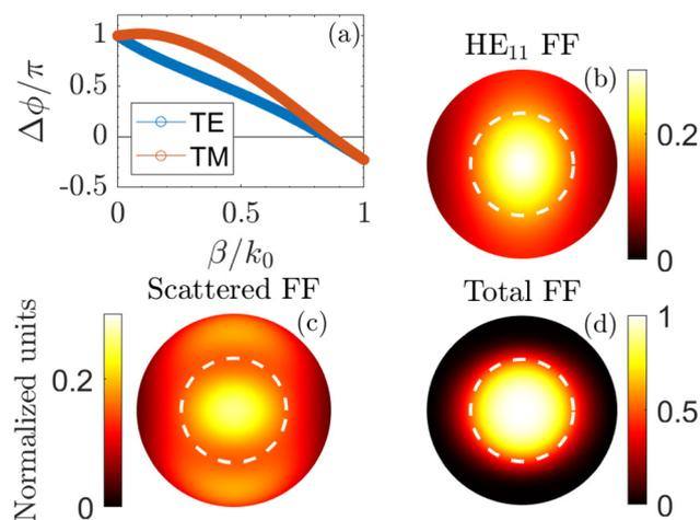
**Fig. 9** (a) The phase difference between the direct transmission of the fundamental mode and the background continuum for TE and TM modes as a function of the propagation constant,  $\beta/k_0$ . (b) The far-field of the fundamental mode. (c) The far-field of the background continuum. (d) The total far-field. The white dotted line indicates NA = 0.75. Be aware of the different color scales that have been used for the far-fields.
