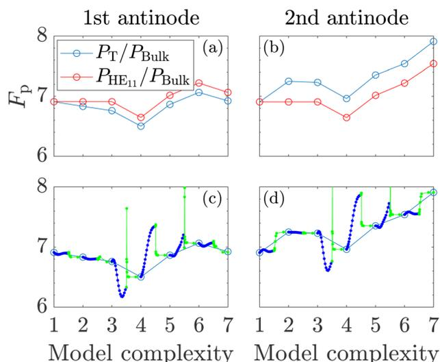
Fig. 11 Purcell factor ( $P_T/P_{\text{Bulk}}$ ) and fundamental mode enhancement ( $P_{\text{HE}_{11}}/P_{\text{Bulk}}$ ) for the 1st (a) and 2nd (b) antinode as a function of the model complexity progression. In (c) and (d) the background continuum is continuously included between each model complexity.
