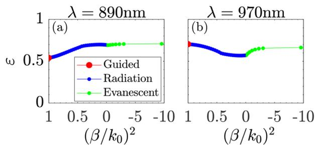
**Fig. 15** Efficiency,  $\varepsilon$  (NA = 0.75), as a function of the initial coefficients expressed with the propagation constant  $(\beta/k_0)^2$  for  $\lambda = 890$  nm (a) and  $\lambda = 970$  nm (b) at the 2nd antinode.
