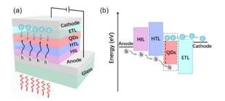
Fig. 1 (a) Schematic illustration of QLEDs with the traditional structure. (b) Energy band diagram of QLEDs and the schematic illustration of charge injection and charge recombination in QLEDs.
