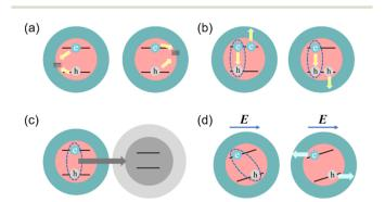
Fig. 4 Schematic illustration of exciton quenching processes. (a) Trapassisted recombination; (b) Auger recombination; (c) energy transfer to non-emissive QDs: (d) field-induced reduction in the overlap between electron wavefunctions and field-induced disassociation.
