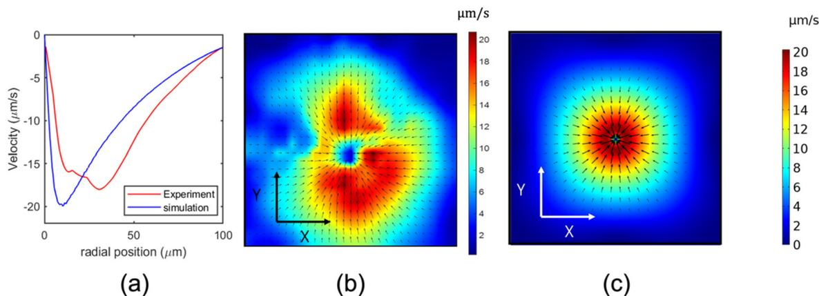
**Fig. 3** ETP results for an illumination intensity of  $11.4 \text{ mW } \mu\text{m}^{-2}$  (a) Radial velocity magnitudes for (b) and (c). (b) Experimental ETP velocity plot in the XY plane generated using particle image velocimetry (PIV) analysis showing radial velocities exceeding  $20 \text{ } \mu\text{m s}^{-1}$  for a 10 V, 20 kHz applied AC. (c) FEM simulation for the ETP flow in the XY plane at  $Z = -2.3 \text{ } \mu\text{m}$  for a 10 V, 20 kHz applied AC.
