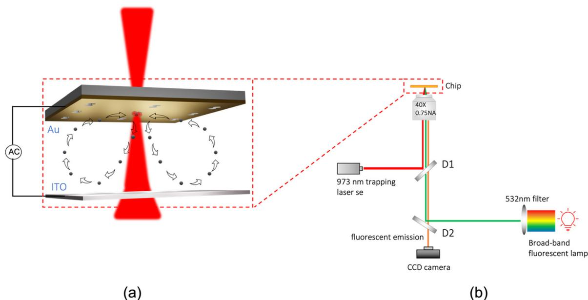
**Fig. 1** Schematic diagram and experimental setup. (a) Schematic diagram showing rapid electrothermoplasmonic (ETP) enabled transport of 25 nm polystyrene spheres towards the plasmonic hotspot. The illuminated double nanohole generates temperature gradients which induce an ETP flow upon the application of an AC field. (b) Experimental setup. D1 and D2 represent dichroic mirrors.
