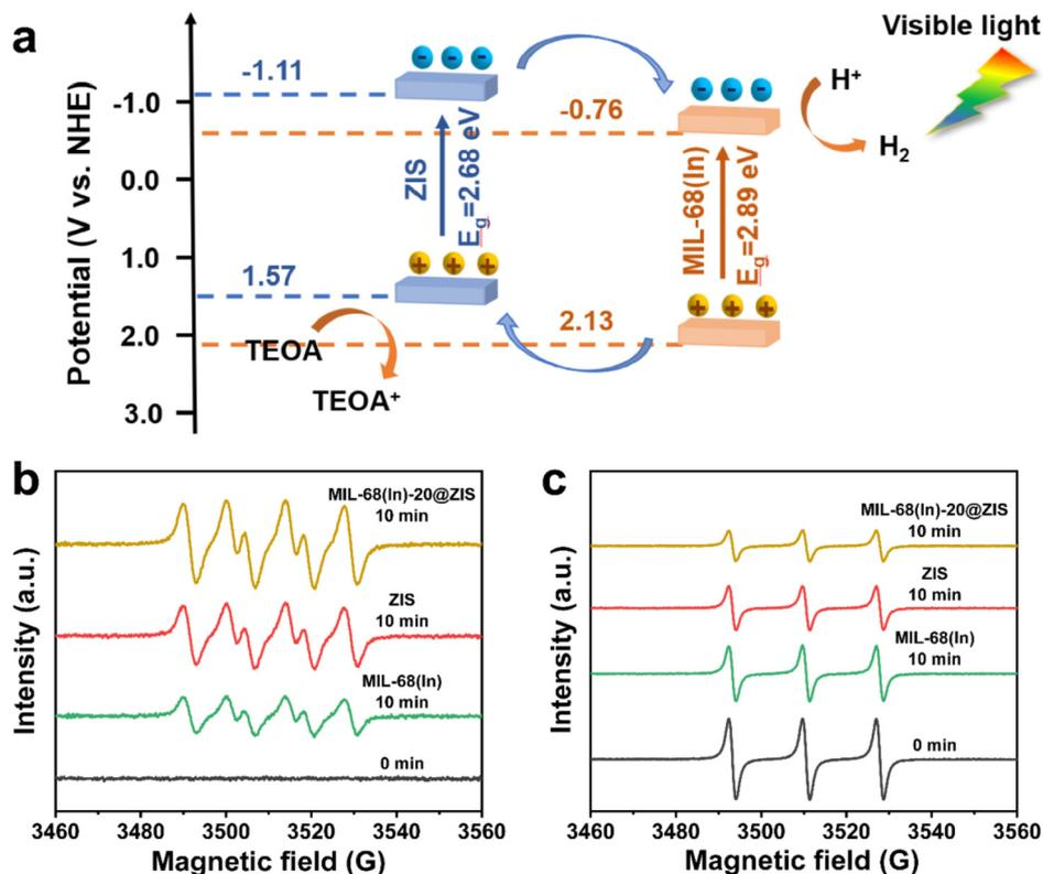
Fig. 6 The photocatalytic mechanism of MIL-68(In)@ZIS. (a) schematic illustration of charge transfer paths for MIL-68(In)@ZIS; EPR spectra of (b) DMPO  $\cdot\text{O}_2^-$  and (c) TEMPO  $\text{h}^+$  for ZIS, MIL-68(In) and MIL-68(In)-20@ZIS.
