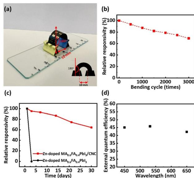
**Fig. 6** (a) Schematic of the bending test of the paper photodetector. (b) Stability of the paper photodetector after various bending cycles. (c) Stabilities of the paper and bare Zn-doped  $\text{MA}_{0.6}\text{FA}_{0.4}\text{PbI}_3$  photo-detectors under ambient conditions. (d) EQE of the paper photo-detectors under 450 nm, 520 nm, and 650 nm laser irradiation.
