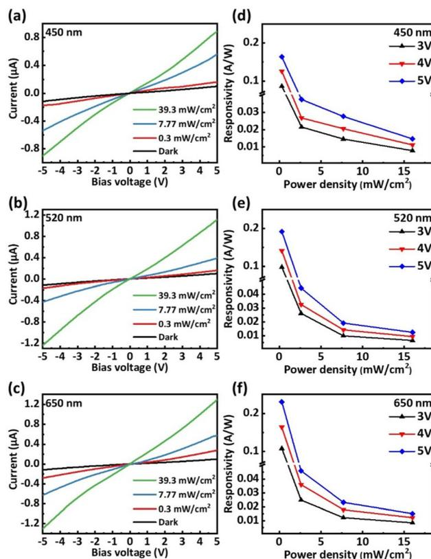
**Fig. 4** *I*-*V* curves of the paper photodetector under dark and light illumination conditions at (a) 450 nm, (b) 520 nm, and (c) 650 nm laser irradiation. Power density dependent responsivity of the paper photodetector under (d) 450 nm, (e) 520 nm, and (f) 650 nm laser irradiation.
