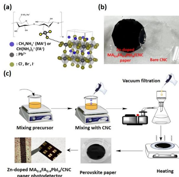
**Fig. 1** (a) Schematic of a Zn-doped MA<sub>0.6</sub>FA<sub>0.4</sub>PbI<sub>3</sub>/CNC structure. (b) Photographic images of bare CNC and Zn-doped MA<sub>0.6</sub>FA<sub>0.4</sub>PbI<sub>3</sub>/CNC papers. (c) Experimental procedure and photograph of the paper photodetector.
