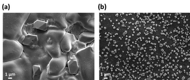
**Fig. 3** (a) SEM image of the Zn-doped MA<sub>0.6</sub>FA<sub>0.4</sub>PbI<sub>3</sub> film. (b) SEM image of the Zn-doped MA<sub>0.6</sub>FA<sub>0.4</sub>PbI<sub>3</sub>/CNC paper.
