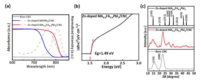
Fig. 2 (a) Absorbance spectra of bare CNC, Zn-doped  $MA_{0.6}FA_{0.4}PbI_3/CNC$ , and Zn-doped  $MAPbI_3/CNC$  papers and fluorescence spectra of Zn-doped  $MA_{0.6}FA_{0.4}PbI_3/CNC$  and Zn-doped  $MAPbI_3/CNC$  papers (dashed lines). (b) Tauc plot of the Zn-doped  $MA_{0.6}FA_{0.4}PbI_3/CNC$  paper. (c) XRD patterns of bare CNC, Zn-doped  $MA_{0.6}FA_{0.4}PbI_3/CNC$  papers, and Zn-doped  $MA_{0.6}FA_{0.4}PbI_3$  films.
