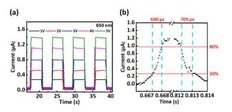
Fig. 5 (a) Time response at various applied voltages under 650 nm laser irradiation. (b) I-t curve of the paper photodetector in a cycle.
