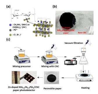
Fig. 1 (a) Schematic of a Zn-doped MA<sub>0.6</sub>FA<sub>0.4</sub>PbI<sub>3</sub>/CNC structure. (b) Photographic images of bare CNC and Zn-doped MA<sub>0.6</sub>FA<sub>0.4</sub>PbI<sub>3</sub>/CNC papers. (c) Experimental procedure and photograph of the paper photodetector.
