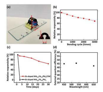
Fig. 6 (a) Schematic of the bending test of the paper photodetector. (b) Stability of the paper photodetector after various bending cycles. (c) Stabilities of the paper and bare Zn-doped MA<sub>0.6</sub>FA<sub>0.4</sub>PbI<sub>3</sub> photodetectors under ambient conditions. (d) EQE of the paper photodetectors under 450 nm, 520 nm, and 650 nm laser irradiation.
