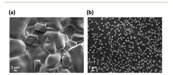
Fig. 3 (a) SEM image of the Zn-doped  $MA_{0.6}FA_{0.4}Pbl_3$  film. (b) SEM image of the Zn-doped  $MA_{0.6}FA_{0.4}Pbl_3/CNC$  paper.
