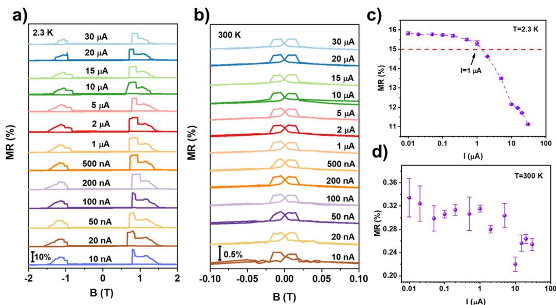
**Fig. 4** Bias-current-dependence of the spin-valve effect in the  $\text{Fe}_3\text{GaTe}_2/\text{MoS}_2/\text{Fe}_3\text{GaTe}_2$  device. MR curves measured at different bias currents from 10 nA to 30  $\mu\text{A}$  at (a) 2.3 K and (b) 300 K. The extracted MR ratios as a function of the bias current at (c) 2.3 K and (d) 300 K.
