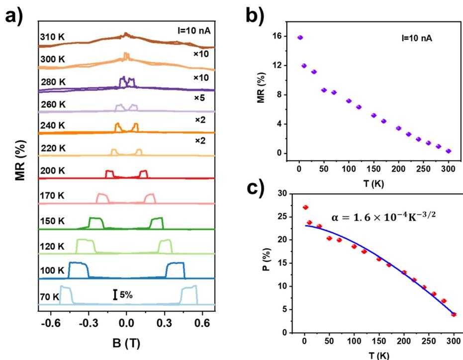
**Fig. 5** Temperature-dependence of the spin-valve effect in the  $\text{Fe}_3\text{GaTe}_2/\text{MoS}_2/\text{Fe}_3\text{GaTe}_2$  device. (a) MR curves measured at different temperatures from 70 K to 310 K with a fixed bias current of 10 nA. (b) The extracted MR ratios as a function of temperature. (c) Spin polarization as a function of temperature. The blue line is the fitting curve according to the Bloch law.
